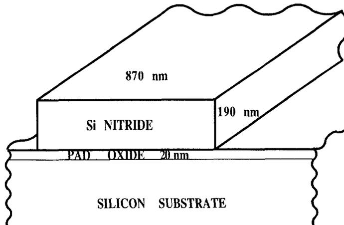
Fig. 3 — Sketch of the geometry of the  $\text{Si}_3\text{N}_4$  line realised by photolithography onto an oxidized silicon substrate.
