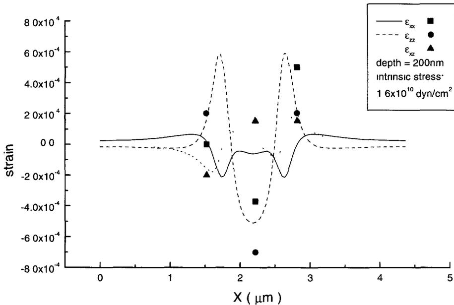
Fig. 4. — Plot of the  $\varepsilon_{xx}$ ,  $\varepsilon_{zz}$  and  $\varepsilon_{xz}$  components of the strain tensor computed by SUPREM IV for the structure shown in Figure 3. The superimposed symbols are the corresponding experimental results deduced from CBED analysis. The abscissa  $x$  is the direction perpendicular to the stripe in the plane of the nitride/oxide interface;  $z$  is perpendicular to the wafer surface.
