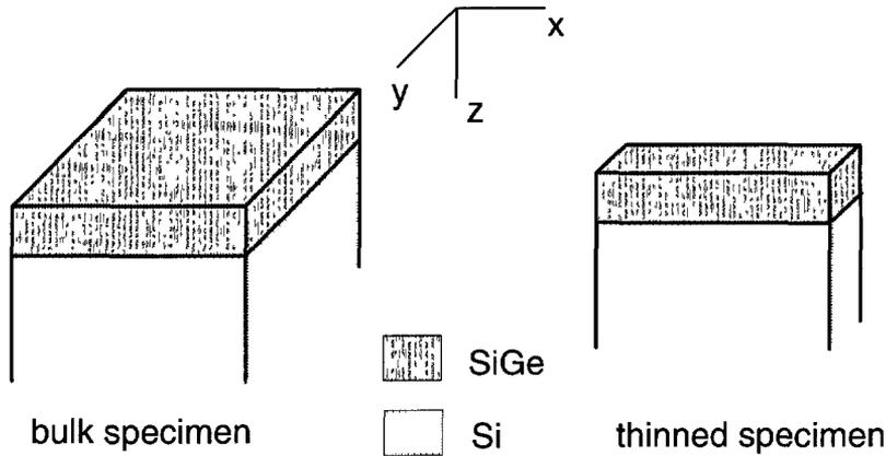
Fig. 1. — Coordinate system chosen in the model for strain relaxation in a TEM specimen.
