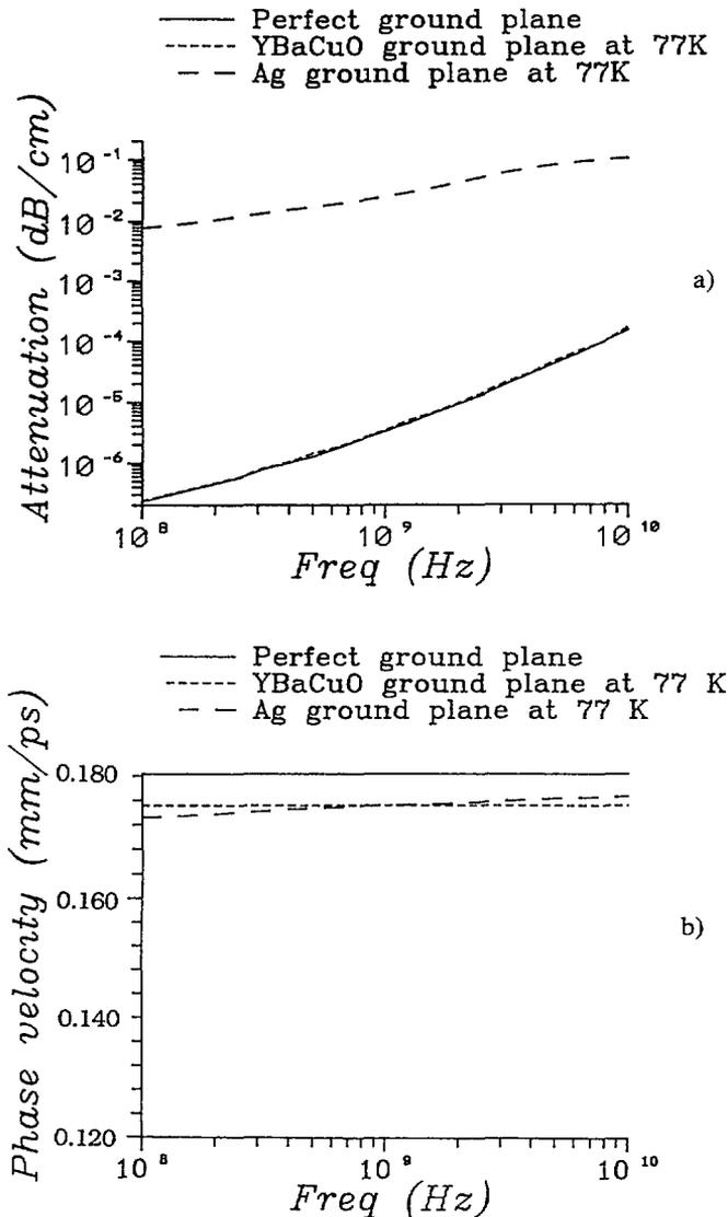
Fig. 6. — Influences of the ground plane on the line attenuation and phase velocity of a superconductive microstrip line.
