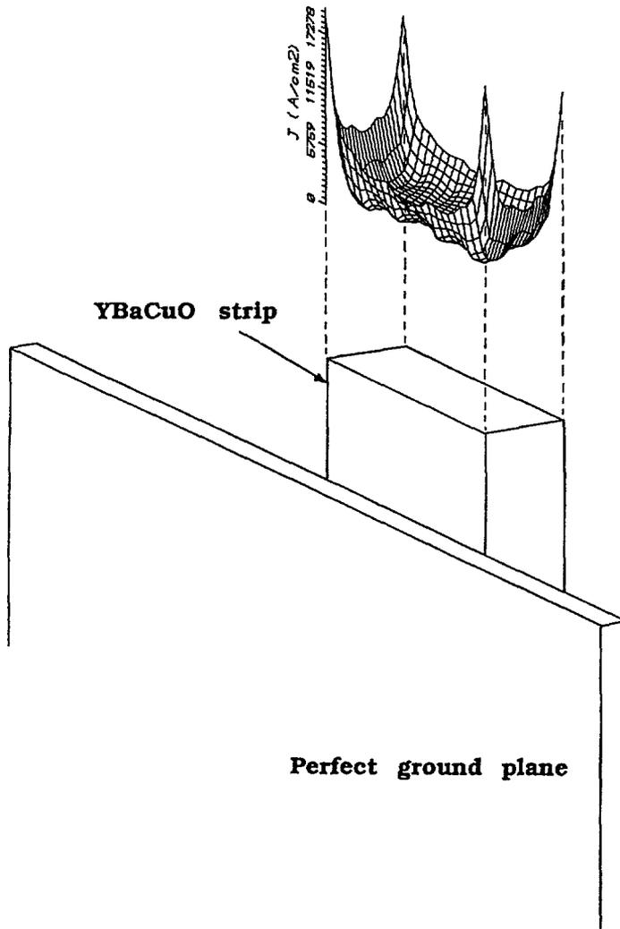
Fig. 8. — Distribution of the current density in the superconductive strip.
