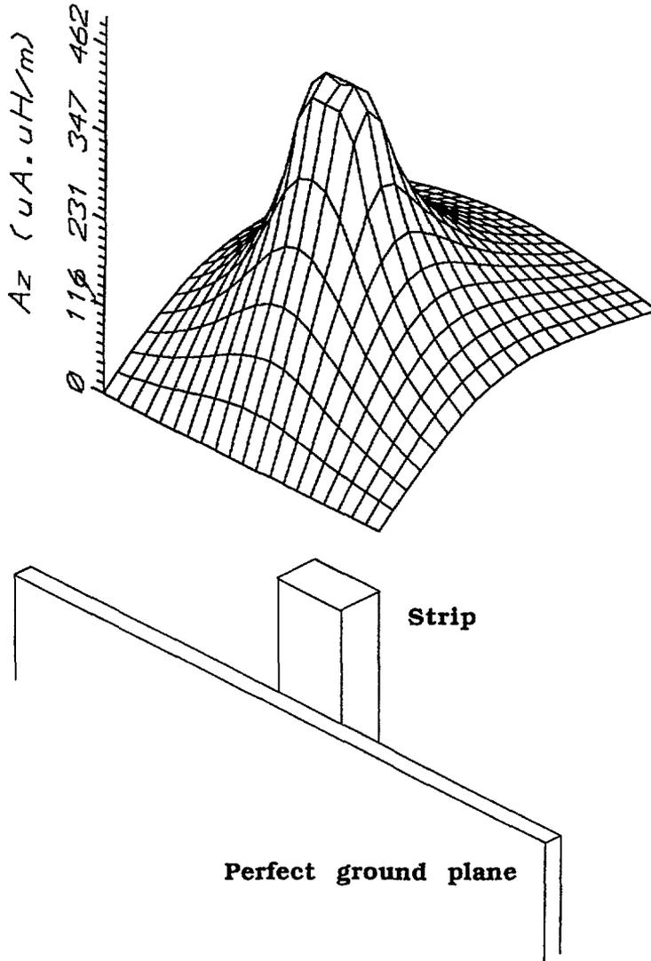
Fig. 4. — Distribution of the potential vector component  $A_z$  in the space.
