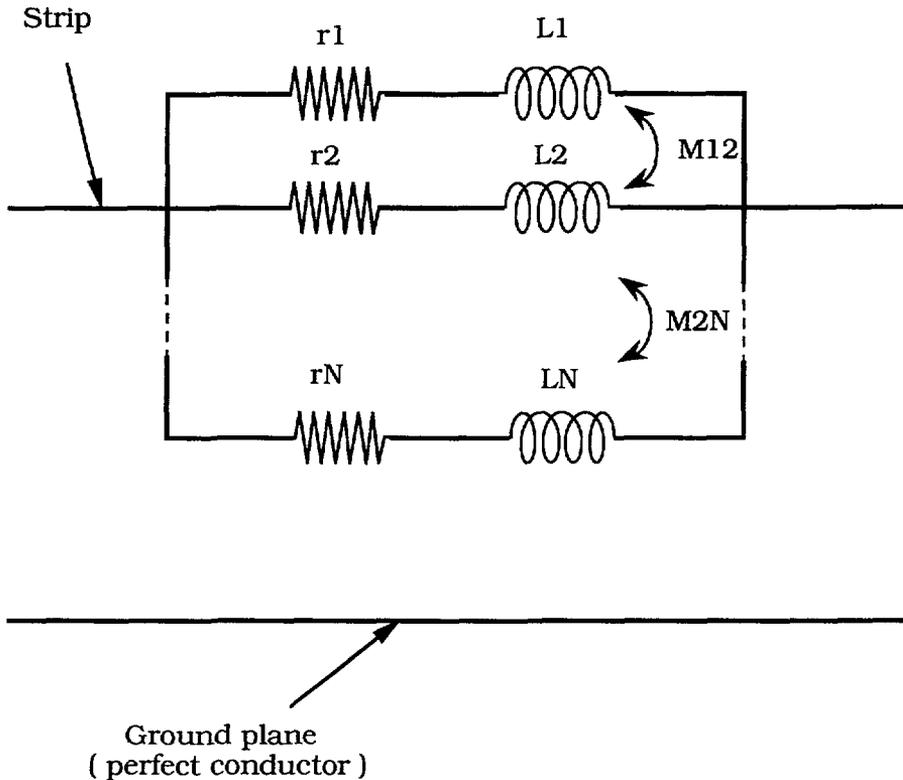
Fig. 2. — Equivalent circuit of the strip.
