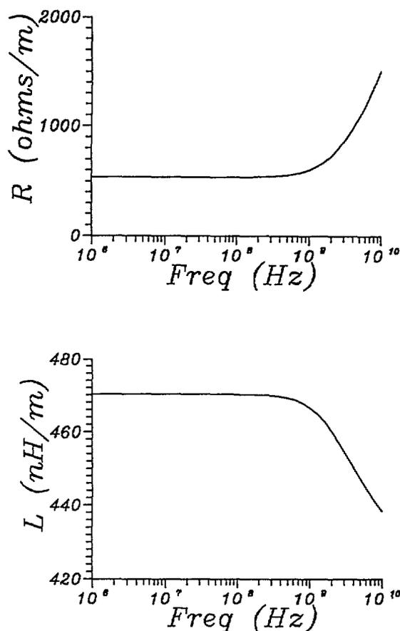
Fig. 3. — The variations of the line resistance  $R(\omega)$  and inductance  $L(\omega)$  versus frequency.
