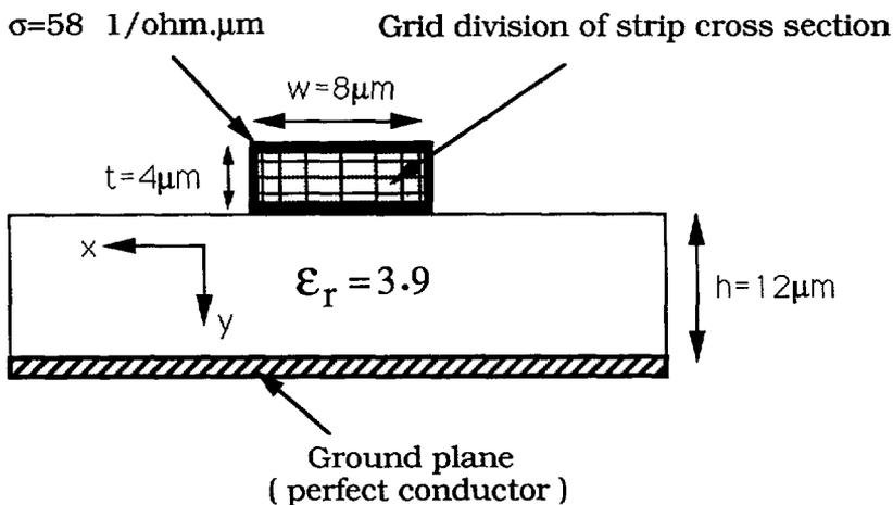
Fig. 1. — Cross section of the microstrip line and its grid division.
