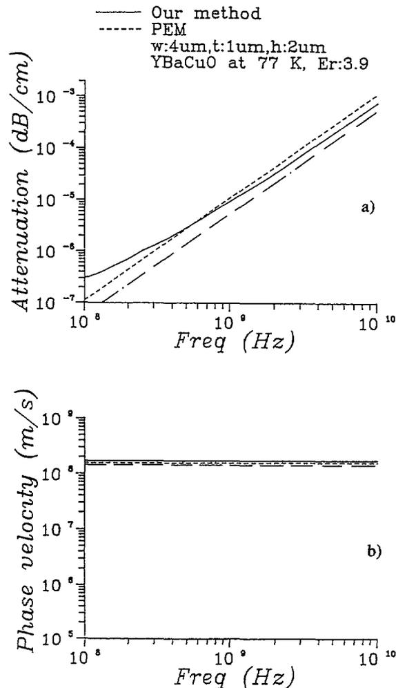
Fig. 7. — Comparison of the variations of attenuation (a) and phase velocity (b) versus frequency, calculated with different methods : (-----) Our method. (... ) Phenomenological Loss Equivalence method. (—) Spectral Domain Approach.
