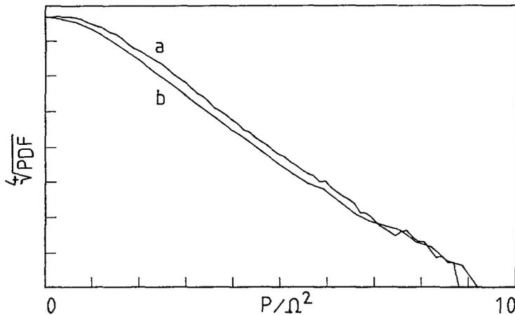
Fig. 5. — Probability density functions of the positive pressure fluctuations to the power 1/4 in the counter-rotating case: (a)  $\Omega_1 = -\Omega_2 = 810$  RPM, (b)  $\Omega_1 = -\Omega_2 = 1250$  RPM. (One unit corresponds to  $0.025 \text{ pa}\cdot\text{s}^2$ ).
