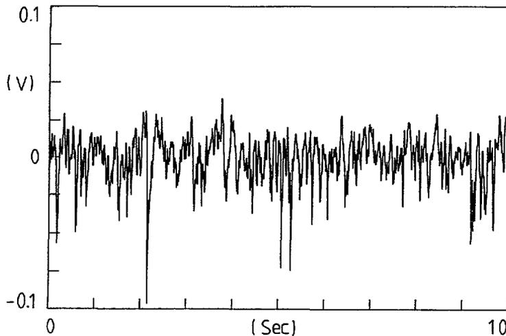
Fig. 3. — Time-recording of pressure fluctuations in the counter-rotating case,  $\Omega_1 = -\Omega_2 = 810$  RPM. (0.1 V corresponds to 2600 pa).
