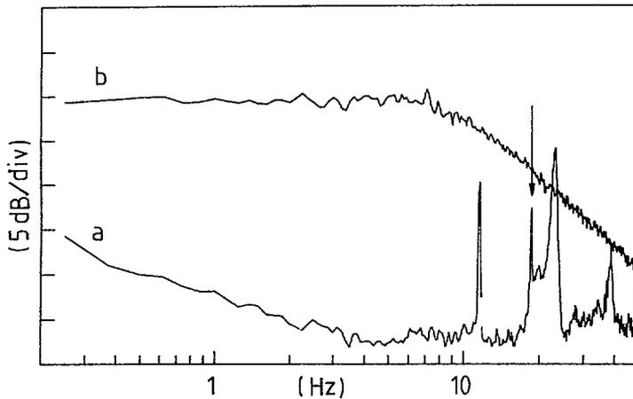
Fig. 2. — Pressure spectra in the co-rotating (a) and counter-rotating (b) cases. For both cases, the absolute value of the rotation rates is 1100 RPM. The peak shown by an arrow corresponds to the rotation frequency. The other peaks correspond to bursting frequencies of the axial vortex generated in the co-rotating case.
