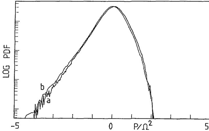
Fig. 4. — Probability density functions of the pressure in the counter-rotating case: (a)  $\Omega_1 = -\Omega_2 = 810$  RPM, (b)  $\Omega_1 = -\Omega_2 = 1250$  RPM. (One unit corresponds to  $0.1 \text{ pa.s}^2$ ).
