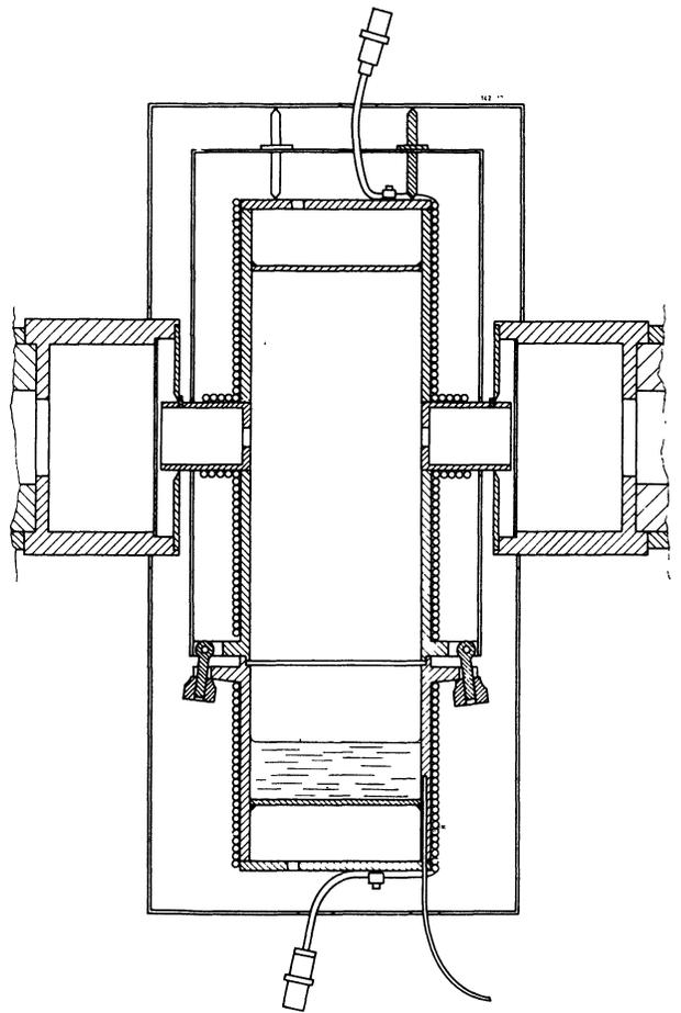
FIG. 2. — Metal vapour charge-exchange cell.
