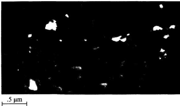
FIG. 3. — 100 kV electron micrograph of as pressed sample; dark field condition.
