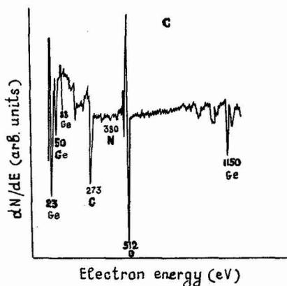
Fig. 4 - Concentration profiles of elements in the subsurface layer of Ge plate after ion-plasma etching (a) and AES spectrum of its surface (b).
