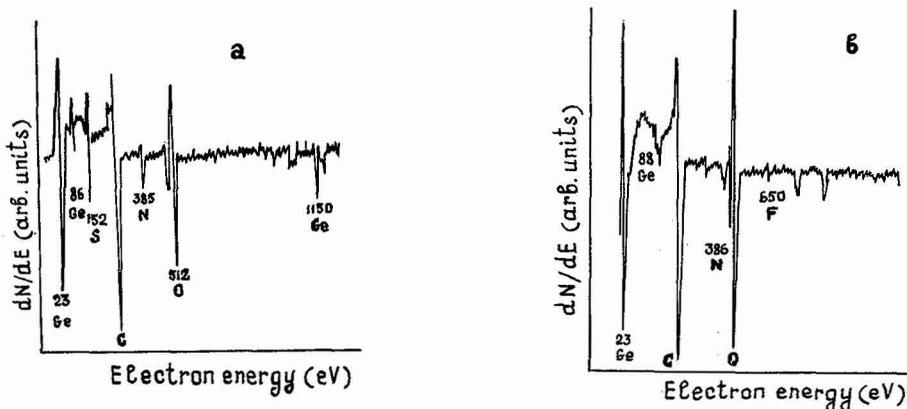
Fig. 3 - AES spectra of Ge plate after the treatment.
