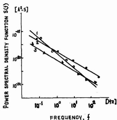
Fig. 6 - Field-emission current fluctuation spectra from semiconductor multi-point arrays taken at  $T = 300$  K in Fowler-Nordheim region of the current-voltage characteristics at emission current
