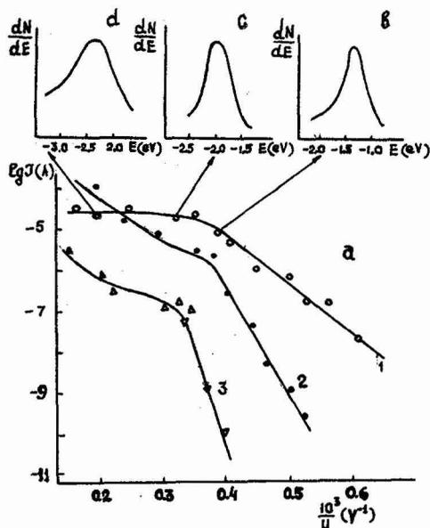
Fig. 5 - a) Current-voltage characteristics of semiconductor multi-point arrays taken at  $T = 300$  K after ion-plasma treatment:
