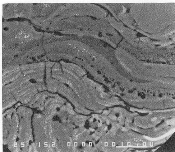
Fig 2. BEI-micrograph showing variation in grey level related to the crack pattern. (bar = 10 \mu\text{m} )
