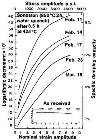
FIG. 1. Ageing at room temperature in laboratory cast SONOSTON (material A) after annealing at 425°C.
