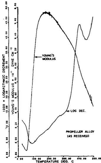
FIG. 3. IF and Young's modulus spectrum of the propeller material measured at a strain amplitude of  $1.25 \times 10^{-5}$ .
