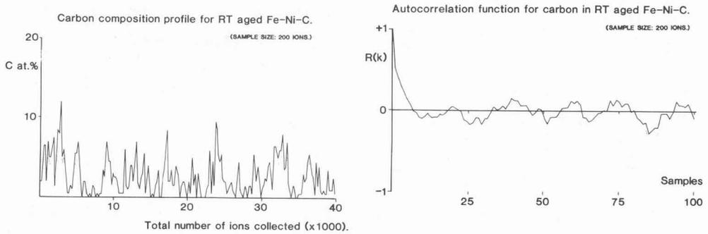
Fig.5 - Composition profile and diagram of autocorrelation analysis after 1870h ageing with original data points averaged over 200 ions.
