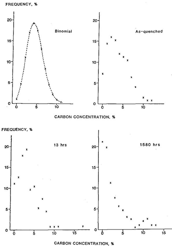
Fig.6 - Frequency distribution of carbon content in 100 ions blocks. Total number of ions collected in each ageing condition was over 10000.
