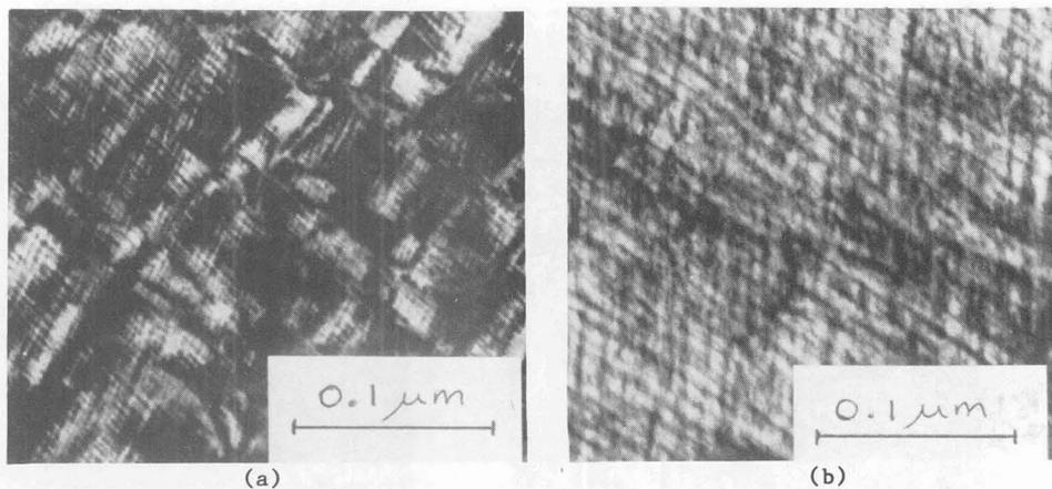
Fig.1 - Electron micrographs of martensite aged at room temperature
