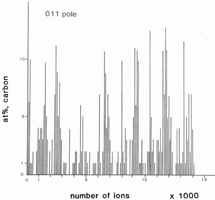
Fig.4 - Composition profile probing through (011) pole with each data point averaged over 100 ions. The specimen was aged for 1580h.
