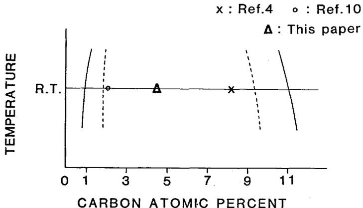
Fig.7 - Schematic phase diagram of spinodal region of martensite. The solid lines are phase boundaries and the dashed lines represent the coherent spinodal.
