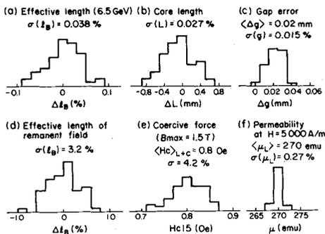
Fig. 2 Statistical distributions of the effective dipole length, fabrication errors and magnetic properties of the silicon steel H23 (S23 grade) for the dipoles.
