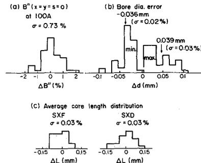
Fig. 6 Statistical distributions of the sextupole strength and fabrication errors.
