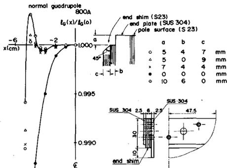
Fig. 3 Radial distributions of the effective quadrupole length after the various end shim corrections for the normal quadrupoles.
