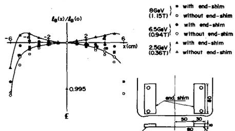
Fig. 1 Radial distributions of the effective dipole length after the end shim correction.
