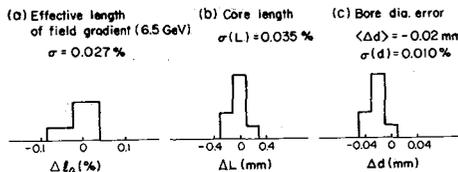
Fig. 5 Statistical distributions of the effective quadrupole length and fabrication errors for the insertion quadrupoles.
