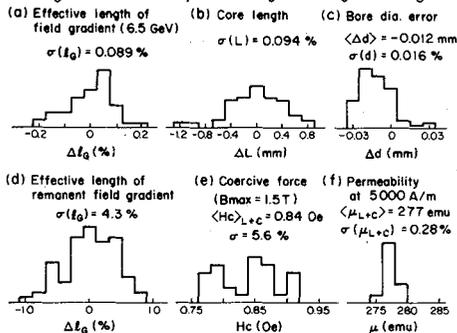
Fig. 4 Statistical distributions of the effective quadrupole length, fabrication errors and magnetic properties of the silicon steel RM23 (S23 grade) for the normal quadrupoles.
