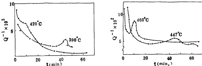
Fig.2 The isothermal internal friction peaks
