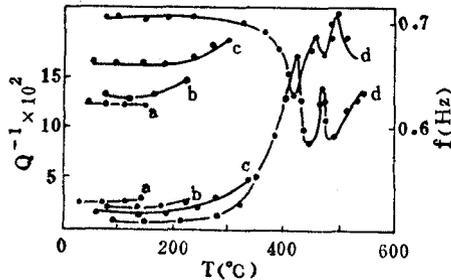
Fig.6 The effect of pre-annealing treatment on structural relaxation
