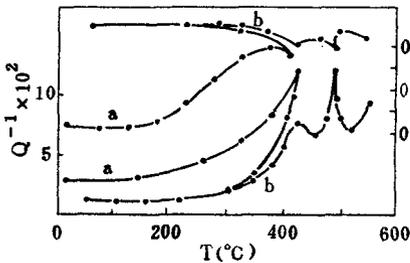
Fig.5 The effect of pre-annealing treatment upto  $425^\circ\text{C}$  on crystallization
