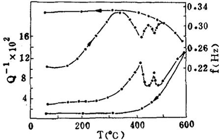
Fig.1 The internal friction and vibrational frequency (heating rate: 5°C/min.)
