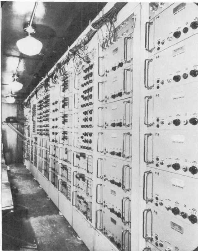
Fig. 6c. Electronics used for selection and recording of neutrino events. Modern electronics would occupy less than one tenth the space.
