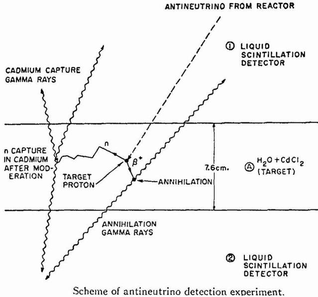
Fig. 5. Schematic of neutrino experiment at Savannah River.
