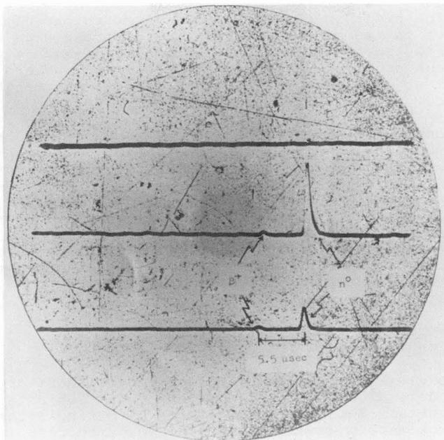
Fig. 6e. A characteristic record. Each of the three oscilloscope traces corresponds to a detector tank. The event recorded occurred in the bottom triad. First seen in coincidence are the positron annihilation gamma-ray pulses in each tank followed in 5.5  $\mu$ sec by the larger "neutron" pulses. A second oscilloscope with higher amplification was operated in parallel to enable measurement of the positron pulses. The positron is denoted by  $\beta^+$  and the neutron by  $n^0$ .
