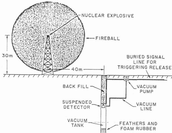
Fig. 1. Scheme for detecting neutrinos from a nuclear explosion.
