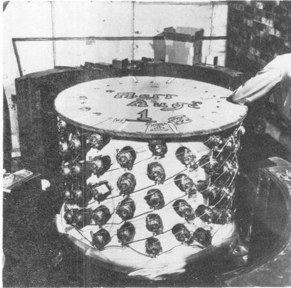
Fig. 3. First large ( $0.3 \text{ m}^3$ ) liquid scintillation detector in shield. The liquid was viewed by 90 2-inch photomultiplier tubes.
