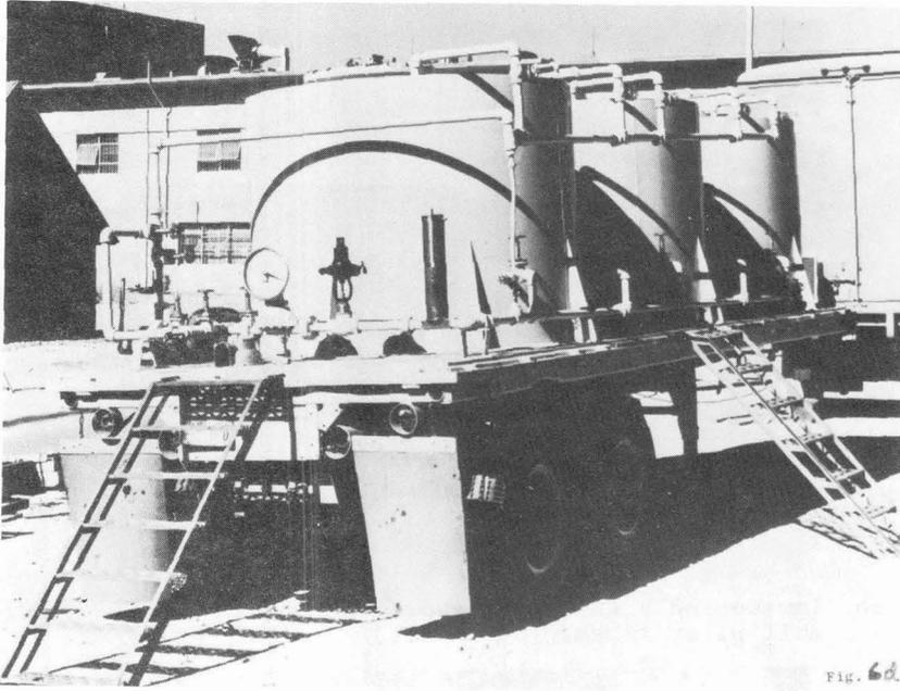
Fig. 6d. The scintillator was stored and shipped in three 1200 gallon steel tanks mounted on a flat bed trailer. The tanks were wrapped with electrical heating strips and covered with fiber glass insulation to keep the scintillator in solution on the trip from Los Alamos to Savannah River.
