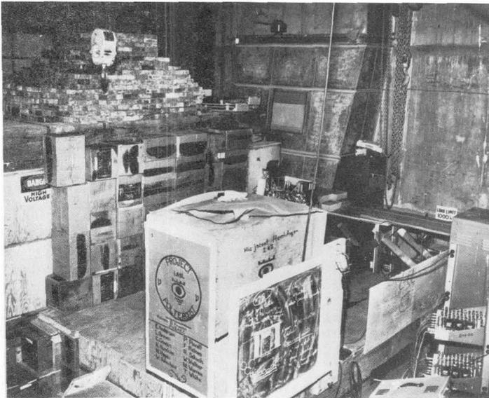
Fig. 4. Shield configuration. The note on the blackboard indicates that we were within a factor of 75 of the required sensitivity. The members of the group for the Hanford Phase of the search are listed on the "Project Poltergeist" sign.
