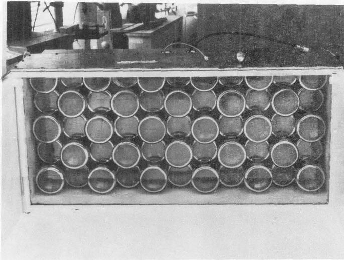
Fig. 6b. Inside end view of detector tank showing 55, 5" photomultiplier tubes.
