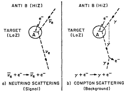
Fig. 8. Schematic of  $\bar{\nu}_e$ ,  $e^-$  detector and discrimination idea.
