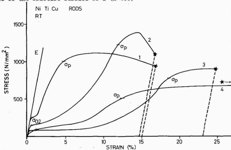
Fig. 2: Stress-stain curves measured at room temperature. Curve 1: c-w specimen, curve 2: specimen c-w and annealed at 300 C; curve 3: specimen c-w and annealed at 500 C; curve 4: annealed specimen (950 C).
