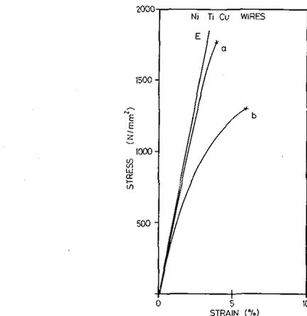
Fig. 5: Stress-strain curves of 2 wires ( $\phi$  0.5 mm) 80 % c-w a and 45 % c-w b.
