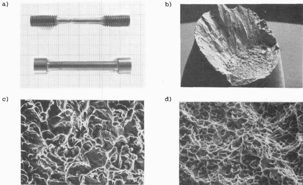
Fig. 1: Photos of the fractured tensile specimens 1 and 4 and of the corresponding fracture surface:
