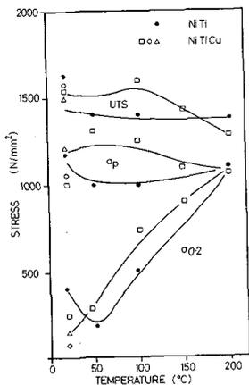
Fig. 3: Yield stress  $\sigma_{0.2}$ , plastic stress  $\sigma_p$  and UTS for NiTi and NiTiCu as a function of temperature.
