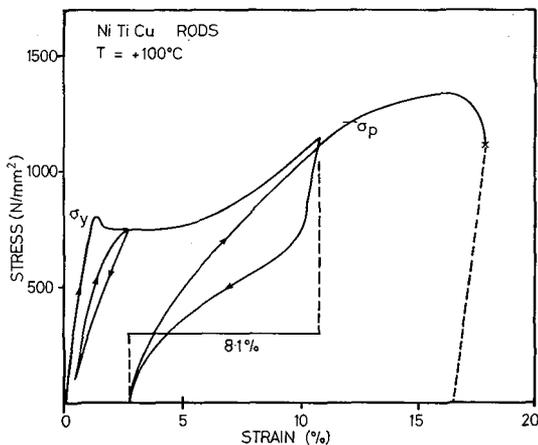
Fig. 4: Stress-strain curve of a NiTiCu specimen measured at 100 C.
