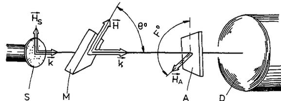
Fig. 1 : Schematic representation of the experiment: S - polarized source, M - transmitter, A - analyser, D - detector.
