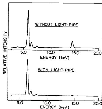
Fig. 10 : Comparison of the X-rays in the 6 keV region and the 14.4 keV  $\gamma$ -ray from  $^{57}\text{Co}$  in copper as observed by an intrinsic Ge detector directly and through a bundled Pyrex low-pass filter. The peak below 5 keV is believed to be an escape peak associated with the 14 keV  $\gamma$ -ray and therefore is reduced with it.
