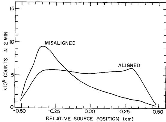
Fig. 4 : Transmission through six sections of 9mm-bore, 115cm long Pyrex vs. transverse position of the source, misaligned and aligned.
