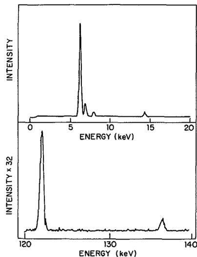
Fig. 11 : The spectra from a  $^{57}\text{Co}$ -in-copper-source observed through a bundle of lead glass capillary tubes. The ordinate for the 120-140 keV region is expanded 32-fold. The transmission at 122 keV is determined from the solid angles subtended by the exit apertures.
