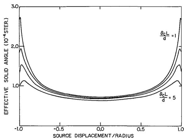
Fig. 8 : The calculated transmission through a circular pipe vs. transverse position of the source for lengths with values of  $\theta_c L/d$  of 1, 2, 3 and 5. The reflection is assumed to be 95% for  $\theta < \theta_c$  and to vanish for  $\theta > \theta_c$ .
