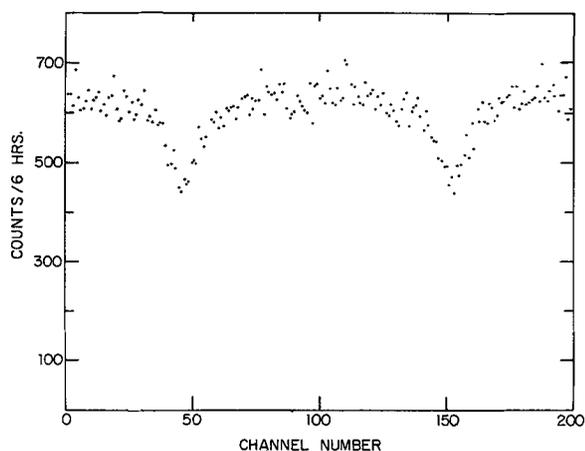
Fig. 7 : Data from a Mössbauer velocity spectrometer for an  $^{57}\text{Fe}$  iron source and absorber with a 7-meter light pipe interposed. A full cycle of the source motion is included and the two resonances observed are the central lines with positive and negative acceleration.
