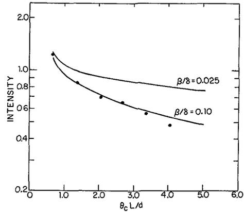
Fig. 6 : Transmission vs. length through the 9mm-bore tubing for a centered source. The solid lines are calculated as in figure 2.
