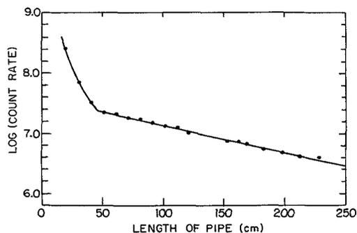
Fig. 3 : Logarithm of the counting rates observed for various lengths of 4 mm-bore Pyrex tubing.
