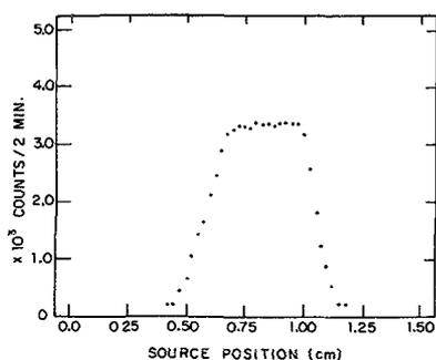
Fig. 9 : The transmission at 6 keV through 2.4m of square glass tubing of 1cm width outside vs. transverse source position.
