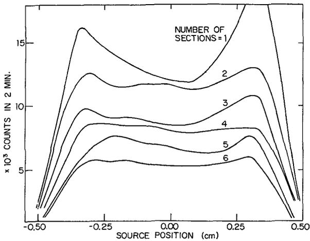
Fig. 5 : Transmission vs. transverse position of the 2mm diam. <sup>57</sup>Fe source for 6, 5, 4, 3, 2 and 1 lengths of 9mm bore, 115cm long, Pyrex.
