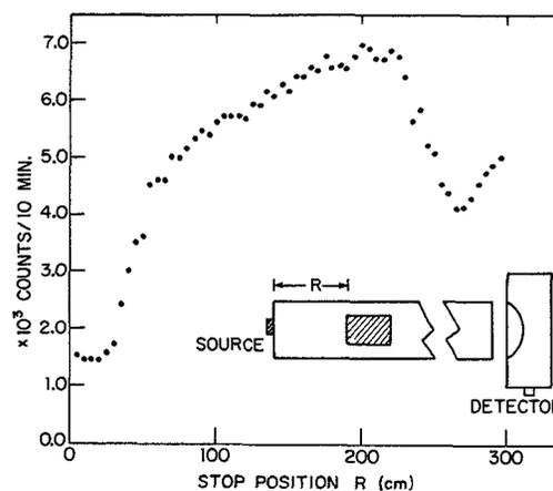
Fig. 12 : Intensity transmitted through a glass pipe from a small source vs. the distance from the source to a cylindrical brass stop. The stop diameter is 8mm and the glass bore is 18mm.
