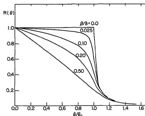
Fig. 1 : The reflection coefficient of intensity  $R(\theta/\theta_c)$  for several values of  $\beta/\delta$ .
