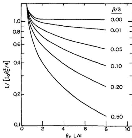
Fig. 2 : Normalized transmission of circular pipes vs. a length parameter  $\theta_c L/d$  for several values of  $\beta/\delta$ .
