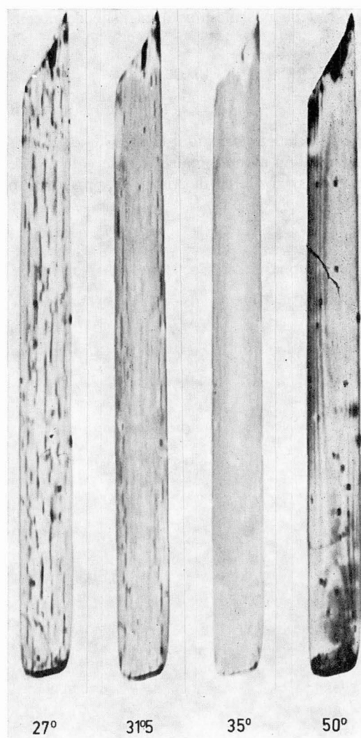
FIG. 1. — Section topographs of the same area of a T. G. S. sample at different temperature. 140 reflection (21 x).
