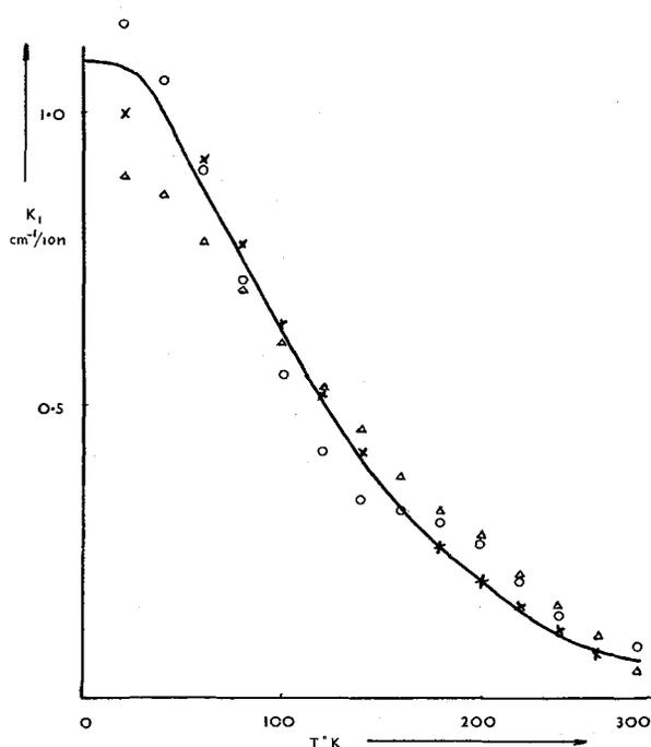
Fig. 3. — Temperature dependence of the cubic anisotropy constant  $K_1$  for Ni<sup>3+</sup> ions on B-sites. ×, lithium doped nickel ferrite with  $x = 0.36\%$ . ○, lithium doped nickel ferrite with  $x = 0.90\%$ . △, nickel excess nickel ferrite with  $x = 0.68\%$ . —, computer fit of the Spin Hamiltonian with the parameters  $g\beta H_{\text{ex}} = 110 \text{ cm}^{-1}$ ,  $\alpha\lambda = -425 \text{ cm}^{-1}$ ,  $\Delta_t = 300 \text{ cm}^{-1}$ .
