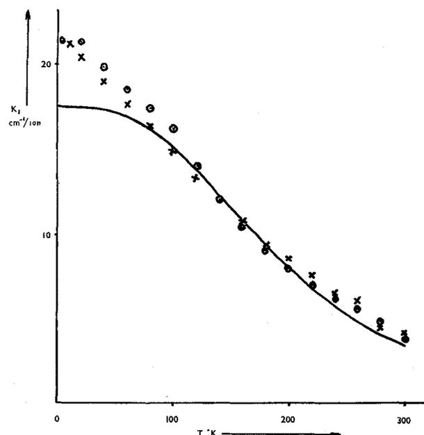
Fig. 4. — Temperature dependence of the cubic anisotropy constant  $K_1$  for Ni<sup>2+</sup> ions on A-sites. ○, pure nickel ferrite water-quenched from 1 220 °C. ×, pure nickel ferrite water-quenched from 1 300 °C. —, computer fit of Spin Hamiltonian with parameters  $g\beta H_{\text{ex}} = 475 \text{ cm}^{-1}$ ,  $\alpha\lambda = -400 \text{ cm}^{-1}$ ,  $\Delta_t = -1 000 \text{ cm}^{-1}$ .
