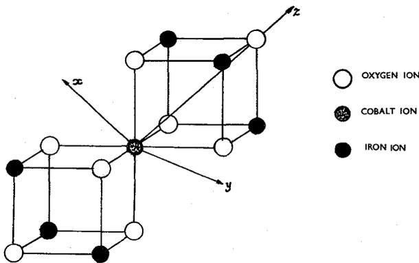
FIG. 1. — Configuration of cations neighbouring a Co<sup>2+</sup> ion in the B-sites of the spinel lattice.
