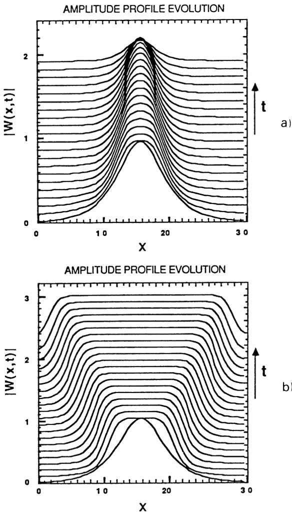
Fig. 2.— 1D pulse-like solution in the case  $\alpha_i = 0$ . Other parameters are  $\mu = -0.1$ ,  $\alpha_r = 1$ ,  $\beta = 3 + i$ ,  $\gamma = -2.75 + i$ , interval length :  $L = 30$ ; a) amplitude profile  $|W(x)|$ ; b) phase profile  $\phi(x) = \arg W(x)$ .
