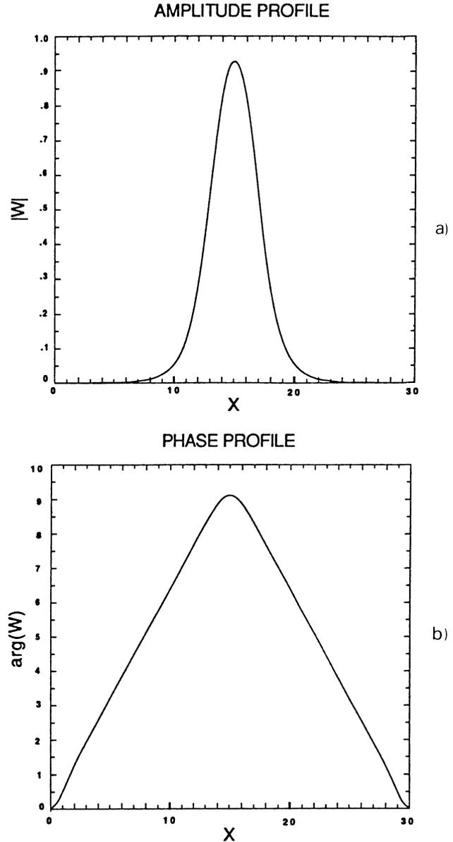
Fig. 3.— Time evolution of a pulse in the variational case :  $\alpha = 1 + 4i$ ,  $\beta = 13.33 + 4i$ ,  $\gamma = -10 + 4i$ , interval length :  $L = 5\pi$ . For these parameter  $\mu_p = -3.33$  ; a) case  $\mu = \mu_p - 0.05$  : the “droplet” shrinks; b) case  $\mu = \mu_p + 0.10$  : the “droplet” grows.
