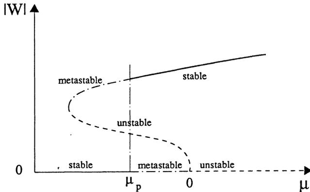
Fig. 1.— Bifurcation diagram of a subcritical Hopf bifurcation. Stationary amplitude  $|W|$  as a function of the control parameter  $\mu$ .
