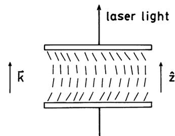
Fig. 1. — The geometry of the sample in the rotatory power experiment. The wave vector of the helical structure is perpendicular to the wall surfaces.
