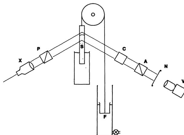
Fig. 1. — Sol-gel film-drawing apparatus and ellipsometer. The reflective silicon substrate S is slowly pulled from a reservoir containing a dilute sol using a hydraulic movement created by a floating cup F on a reservoir draining through a controlled orifice. The ellipsometer consists of a beam expander X, a polarizer P, a  $\lambda/4$  compensator C, an analysing polarizer A, a diffusing screen S and a video camera V. The polarizers are motorized.
