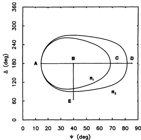
Fig. 3. — Locus of extinctions as function of ellipsometric angles  $\Delta$  and  $\Psi$  (related to polarizer angles) for indexes  $n_1$  and  $n_2$  (solid curves, with  $n_1 < n_2$ ) and spatially varying film index (dashed curve). Motorized polarizers allow searching along paths that guarantee crossing an extinction in the film.
