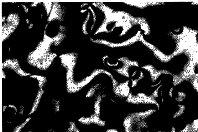
Fig.3.— Optical texture observed for the smectic P phase at 216°C under crossed polars.
