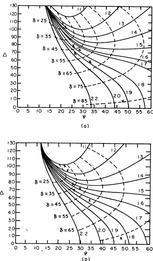
FIG. 3. — Section of the  $\Delta$  vs.  $\psi$  plane with experimental points representing oxidized specimens. Evaluated for (a) ideal Gas As-film interface (b) arsenic film at the interface.
