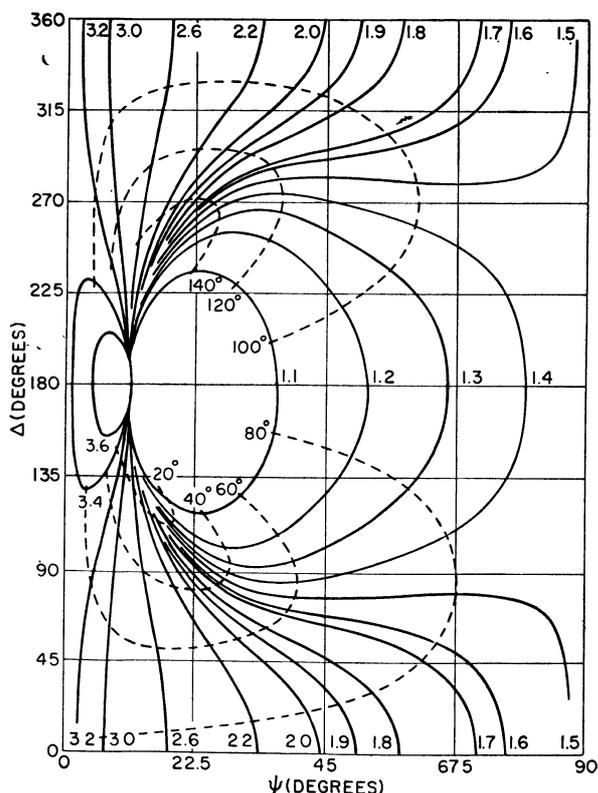
FIG. 2. —  $\Delta$  and  $\psi$  as a function of the index of refraction and thickness of transparent film on GaAs. Full lines are loci of constant index of refraction, dashed lines are loci of constant  $\delta$ .
