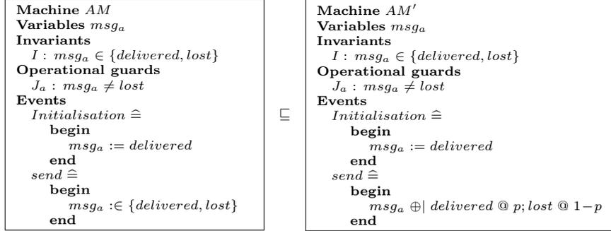
**Fig. 5.** A simple communication protocol: introducing probabilities
