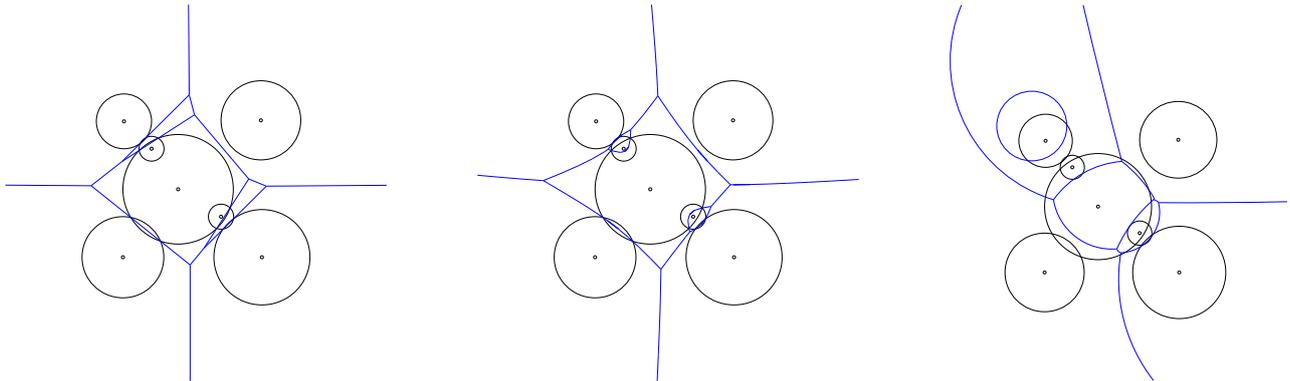
Figure 1: Curved Voronoi diagrams of 7 circles / weighted points. (Left) Power diagram  $d(S_i(c_i, r_i), p) = \|p - c_i\|^2 - r_i^2$ . (Middle) Apollonius diagram :  $d(S_i(c_i, r_i), p) = \|p - c_i\| - r_i$  (Right) Möbius diagram :  $d(S_i(c_i, a_i, r_i), p) = a_i \|p - c_i\|^2 - r_i^2$ .
