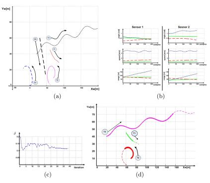
**Fig. 3.** Sensor registration with moving observers and moving targets (a) Simulation environment: O - observer, T - target, (b) Extracted target attributes, *solid line*-target 1, *dashed line* - target 2, *dotted line* - target 3, (c) Learning curve, and (d) All data transformed into sensor 1 reference frame
