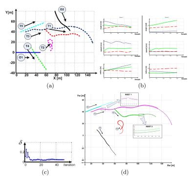
**Fig. 4.** Sensor registration with moving observers and moving targets experiencing occlusions (a) Simulation environment: O - observer, T - target, (b) Extracted target attributes, *solid line*- target 1, *dashed line* - target 2, *dotted line* - target 3, (c) Learning curve, and (d) All data transformed into sensor 1 reference frame
