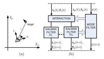
**Fig. 1.** a) Coordinate frames: W- world coordinates, S - sensor coordinates and b) The IMM algorithm [10]:  $\hat{\mathbf{x}}_i$ ,  $\hat{\mathbf{P}}_i$  define the states and their covariance matrices for i = 1, ..., N hypotheses.  $\hat{p}(t)$  is the mode probability
