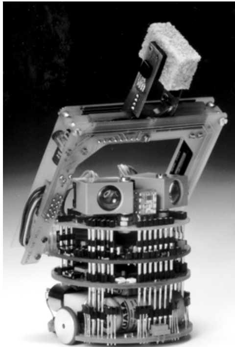
Figure 2: The Khepera mobile robot
