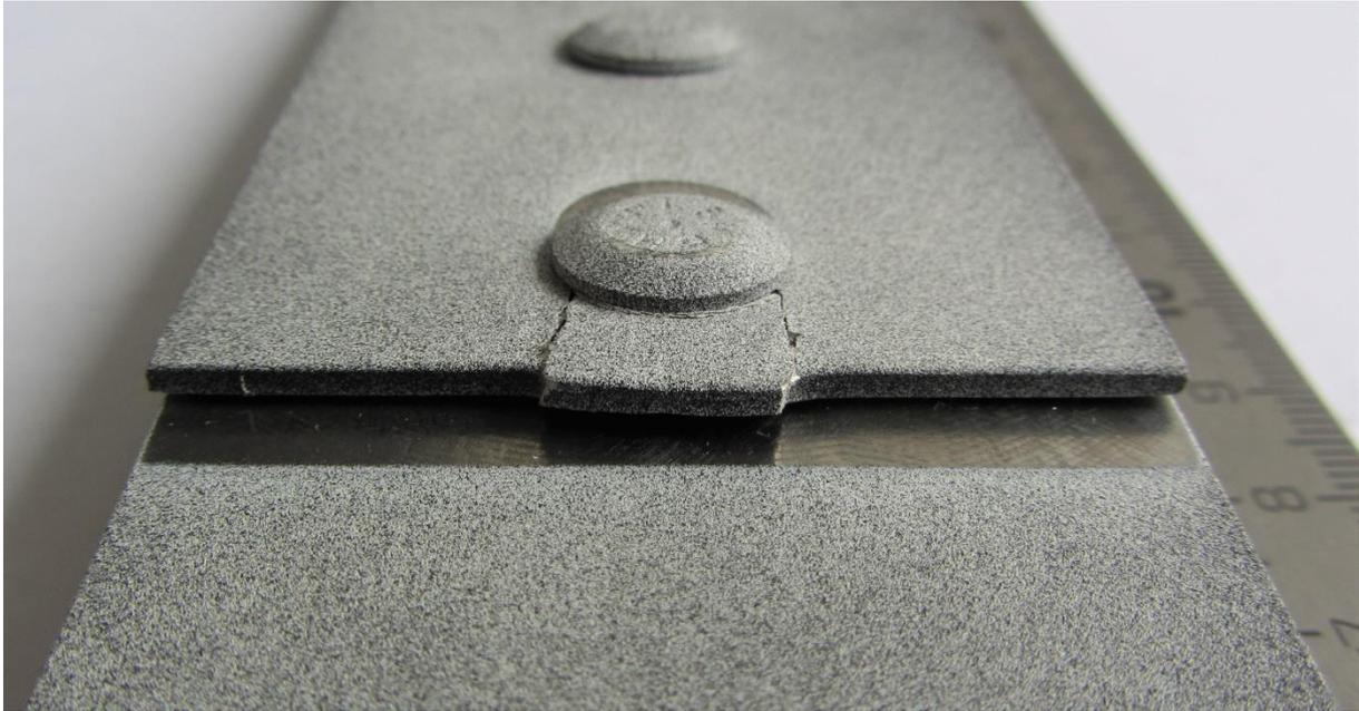
**Figure 18 : Representative failure of a specimen with small thickness**
