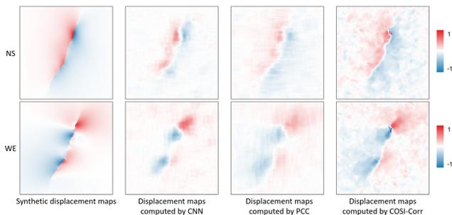
**Fig. 3.** (top) North(red)-South(blue) displacement maps; (bottom) West(red)-East(blue) displacement maps for the CNN, PCC, and COSI-Corr approaches.
