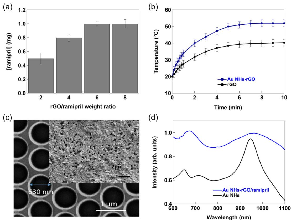
**Fig. 2** Ramipril loading onto rGO-coated nano-heating elements. (a) Ramipril (1 mg) loading capacity of rGO as a function of rGO/drug ratio. (b) Photothermal heating curves of water using rGO directly deposited on Kapton or on a nano-heater in the form of Au NHs. (c) SEM image of Au NHs without and upon coating with rGO/ramipril (inset). (d) UV-Vis absorption spectra of Au NHs and Au NHs-rGO/ramipril in air.
