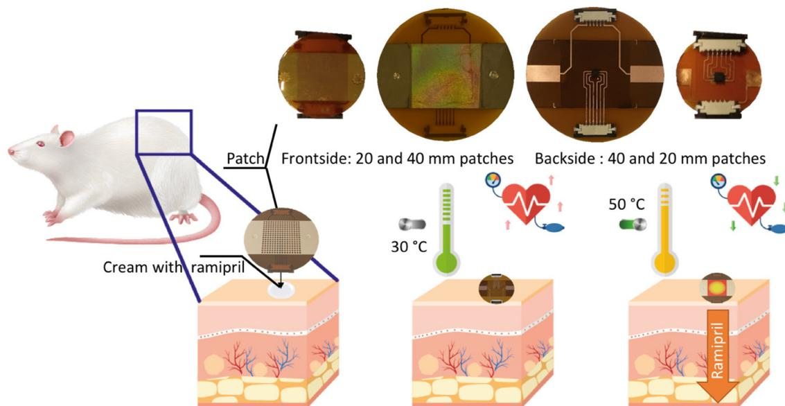
**Fig. 1** *In vivo* model for electrothermal ramipril delivery. Enhanced ramipril permeation upon combination of nano-engineered heating elements with a transdermal vehicle, Pentravan® loaded with ramipril (10%).
