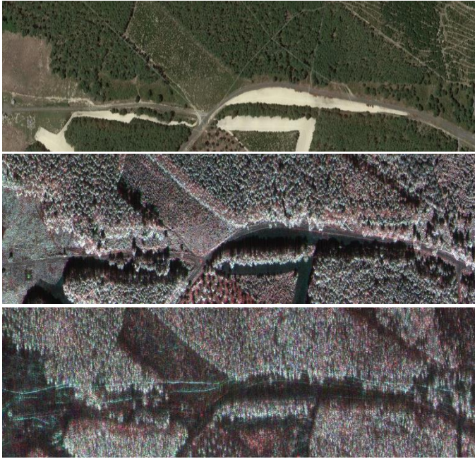
Fig. 8. Optical (up), multi-temporal X (middle) and VHF-UHF (down) band images of buried cables.
