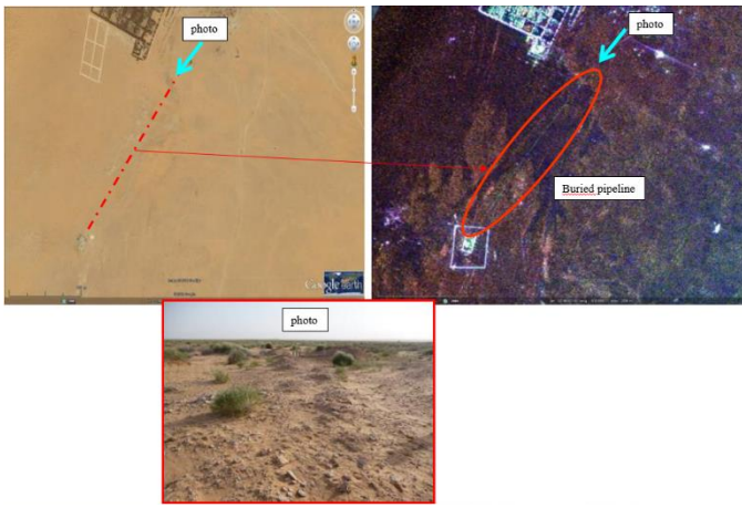
Fig. 2. Zoom of full polarized VHF-UHF Band (right) and optical (left) images on pipeline detection, and photo of corresponding ground (down)
