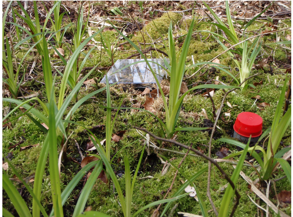
Figure 5 In the spring of 2012 fifteen pitfall traps were placed at the site, consisting of a container with some preservative buried in the ground and a rain cover placed on top. Next to each pitfall a groundwater monitoring well was placed for abiotic measurements. Photo Rink Wiggers.
