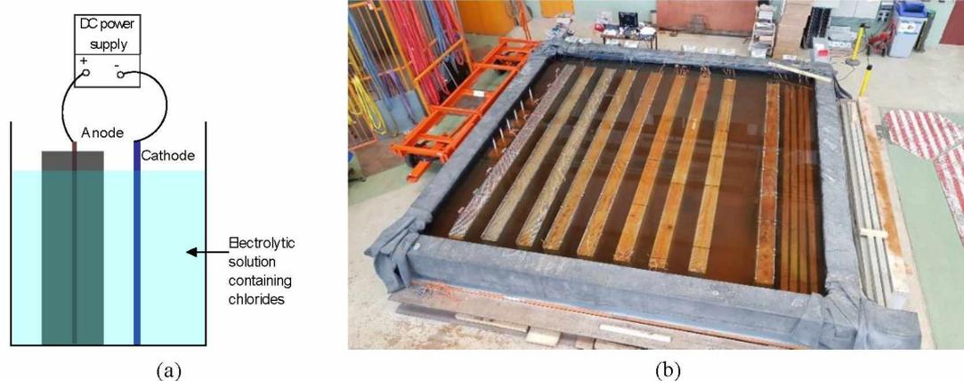
Figure 2: Accelerated corrosion technique: (a) Simplified setup, (b) Corrosion of the specimens.
