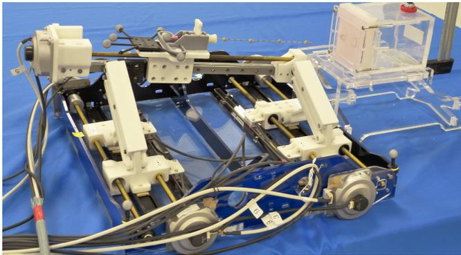
Fig. 15: Set-up used to determine the accuracy of needle tip pose during the insertion.
