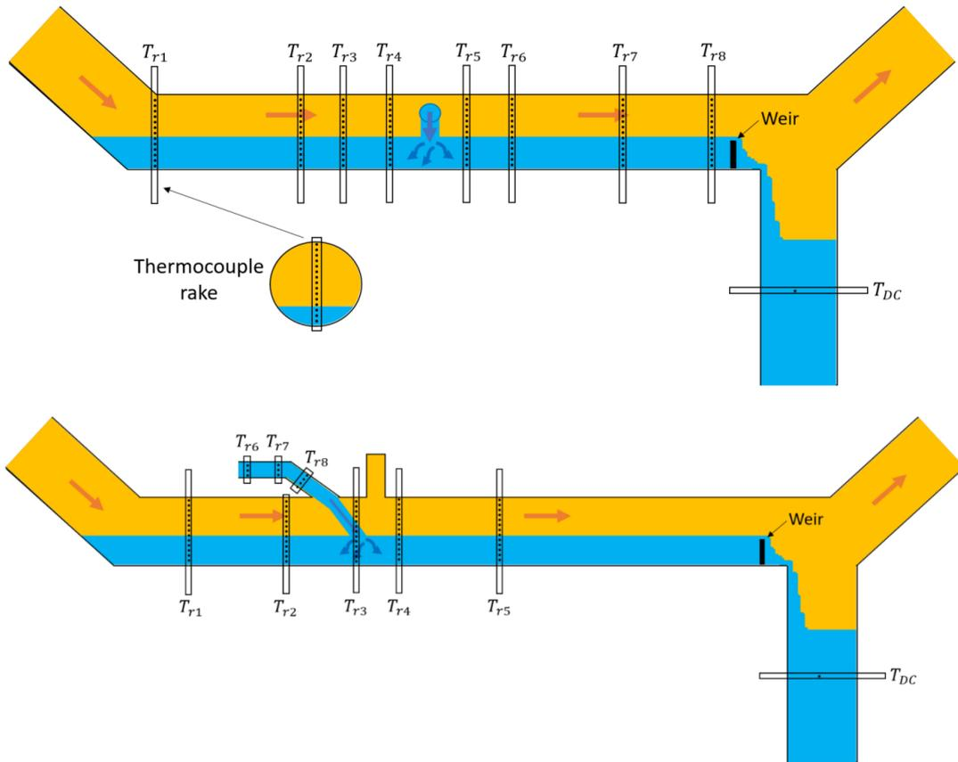
**Fig. 3** Framatome (at the top) and Westinghouse (at the bottom) test sections in the COSI experiment.
