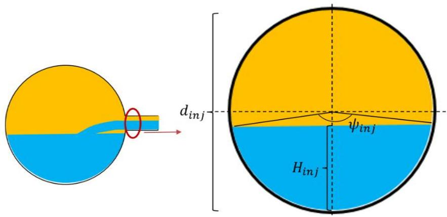
**Fig. 12** Stratified flow in the UPTF injection pipe.
