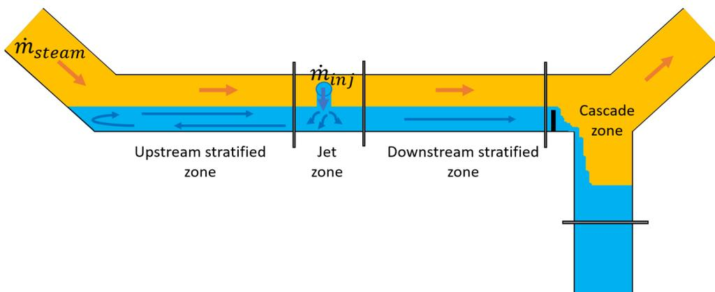
**Fig. 5** Phenomenology in the COSI test section.
