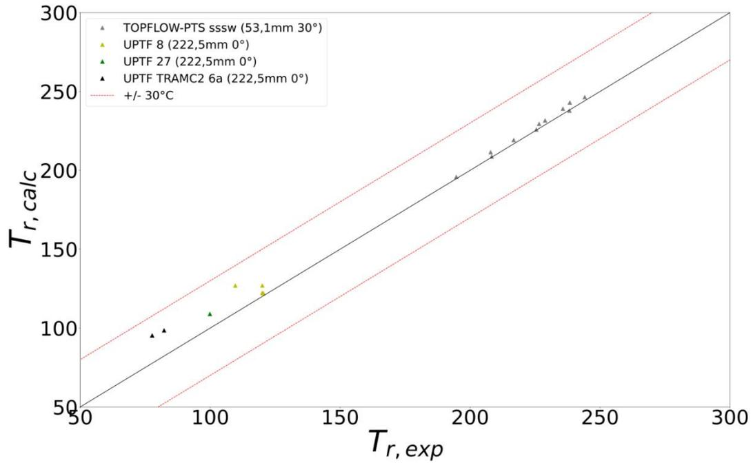
**Fig. 25** Prediction of the mean liquid temperature against the validation database.
