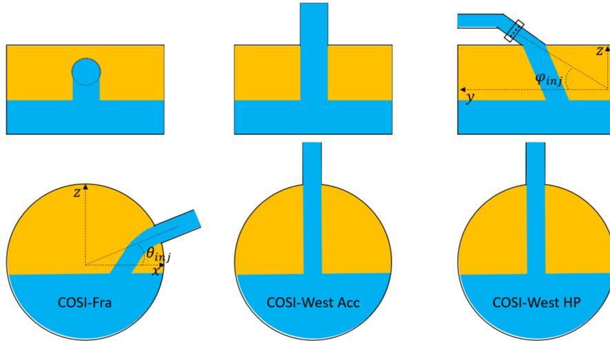
**Fig. 4** Geometrical configurations of the injection pipe in the COSI experiments.
