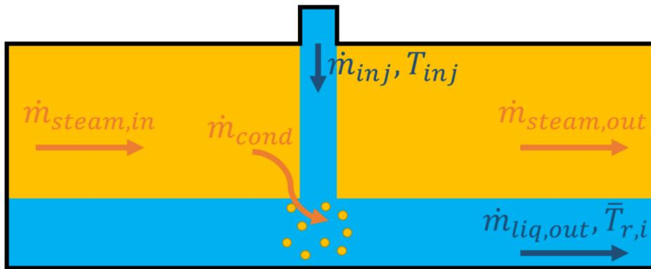
**Fig. 17** Control volume between the injection and a thermocouple rake.
