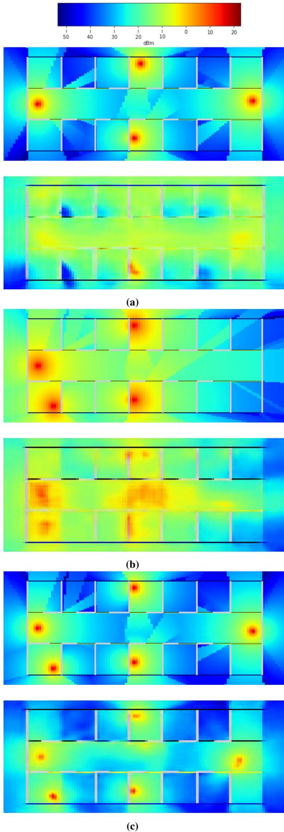
**Fig. 8:** Reconstructed maps (rows 2, 4 and 6) and its corresponding original exposure maps (rows 1, 3 and 5) when (a) 15, (b) 50, (c) 90 pixels used as sensor measurements at random locations.
