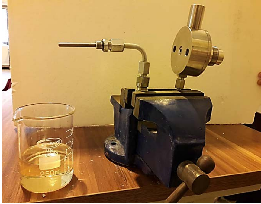
Fig. 3. Turbine meter oil inlet pathway for the velocity measurement system.
