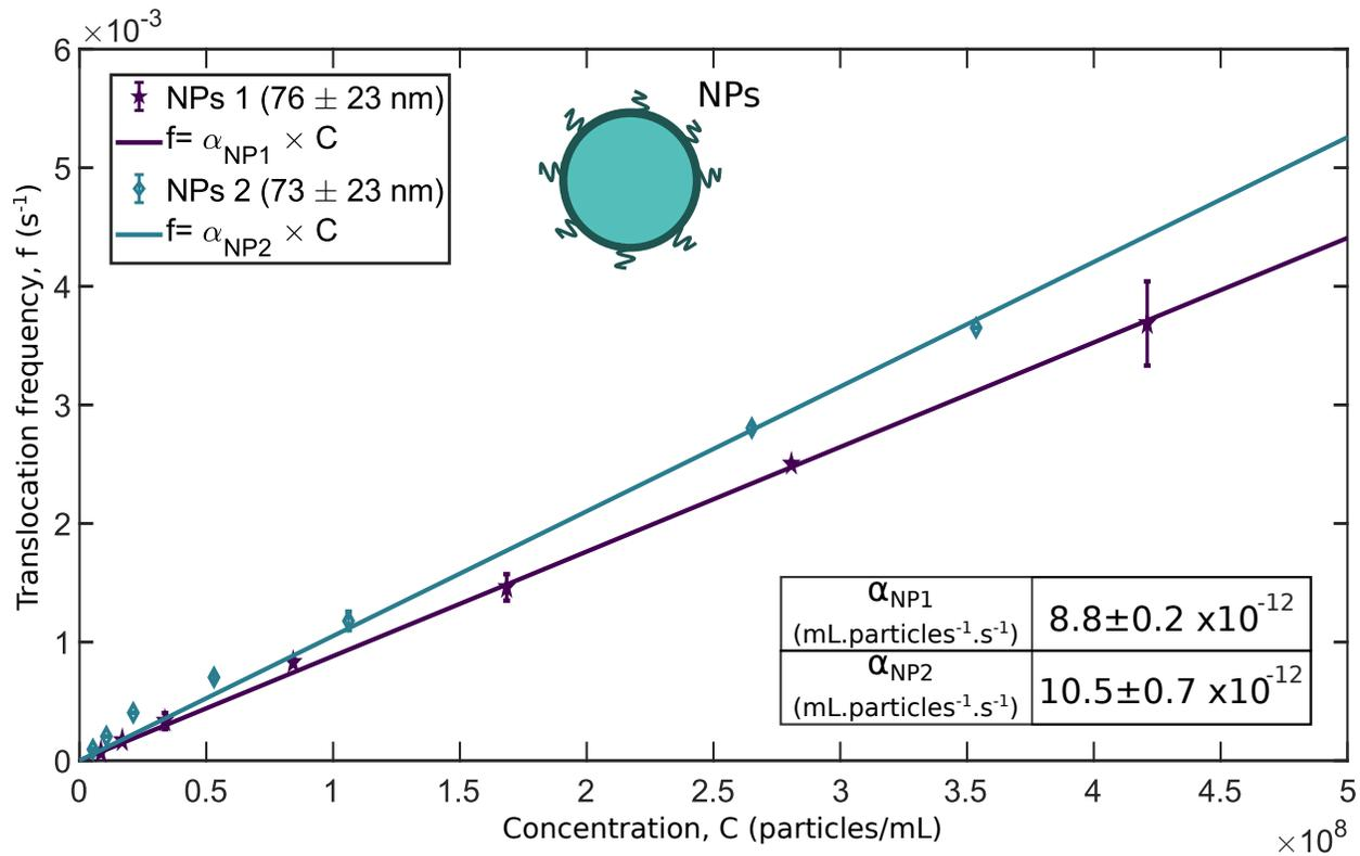
Figure 2: **Calibration of the experimental setup using fluorescent polystyrene nanobeads (NPs).** Translocation frequency ( $f$ ), as a function of NPs concentration ( $C$ ), for two batches of NPs. Continuous blue and violet curves corresponded to linear fit. Pore diameter 400 nm, Applied pressure 0,5. Experimental errors were the standard error of the mean, and  $N_{\text{replica}} > 36$  for each experimental series.
