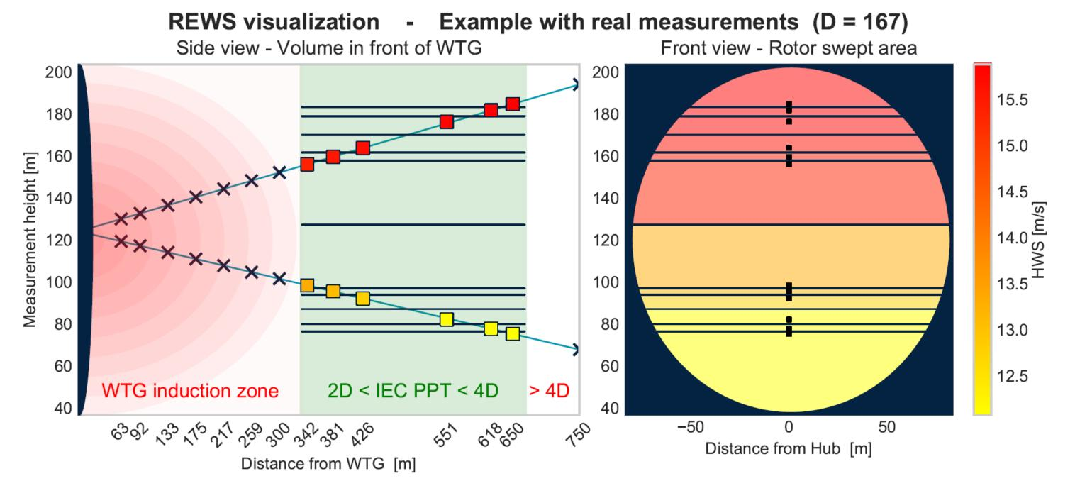
In the example above, the REWS is calculated using 12 HWS measurements at 12 different heights without any assumption on a vertical wind shear profile. Therefore, this implementation relies only on the hypothesis of horizontal flow homogeneity, which assumes that wind speed is homogeneous at a given height. In simple terrain, outside the induction zone and wakes, this hypothesis is reliable and is already in use for both WindCube and WindCube Nacelle.
