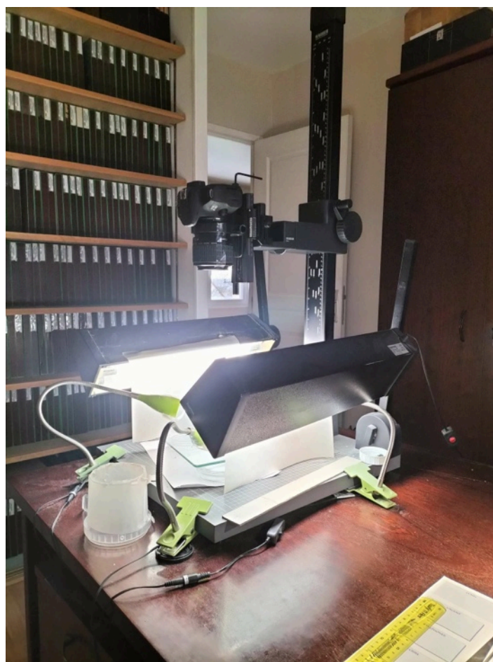
Photo 6. Shooting equipment: Canon 850D case, Canon MPE 65 lens, Sigma 50 Macro lens, Lighting composed of two neon ramps and 4 small LED lamps (Pascal Deschamps).
