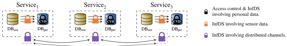
**FIGURE 1** Three services have their own local sensitive personal data protected by an InfDS involving personal data and another involving sensor data. The services collaborate via a last InfDS to be protected against distributed inference attacks
