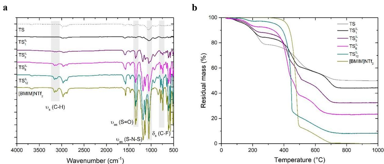
**Figure 3.** (a) FT-IR spectra and (b) TGA curves of P<sup>2</sup>SG monoliths  $\text{TS}_x^{\text{IL}}$  (where x is the initial volume of IL), neat TS monolith and IL.
