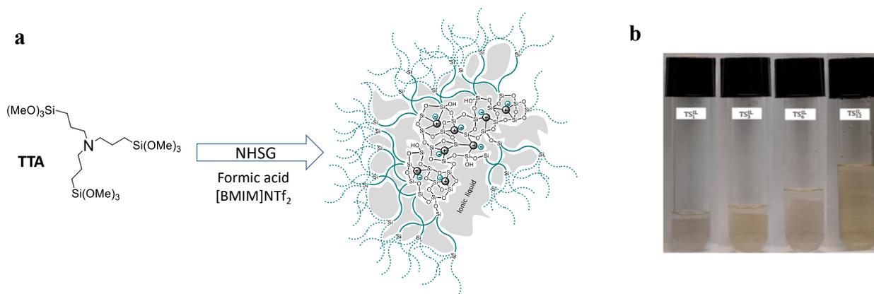
**Figure 1.** (a) Schematic synthesis of ionosilica ionogels; (b) photograph of the ionosilica ionogel monoliths with different IL volumes.
