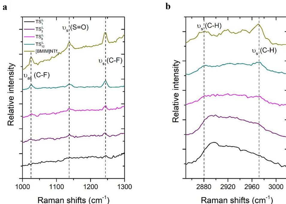
**Figure 6.** Raman spectra of the  $\text{TS}_x^{\text{IL}}$  ground monoliths and the pure IL in the range of (a) 1000-1300  $\text{cm}^{-1}$  and (b) 2850-3100  $\text{cm}^{-1}$ .
