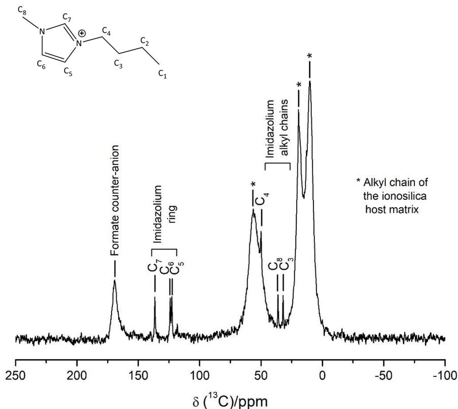
**Figure 2.** Solid-state  $^{13}\text{C}$  CP NMR spectrum of the I<sup>2</sup>SG monolith synthesized in the presence of 6 mL of IL(**TS<sub>6</sub><sup>IL</sup>**). NMR shifts (ppm): TS alkyl chain (9.9, 19.2 and 56.7 ppm); C<sub>3</sub>(32.1 ppm); C<sub>4</sub> (50.1 ppm); C<sub>5</sub> (122.6 ppm); C<sub>6</sub> (123.9 ppm); C<sub>7</sub> (136.4 ppm); C<sub>8</sub> (36.0 ppm) and formate counter-anion (166.7 ppm).
