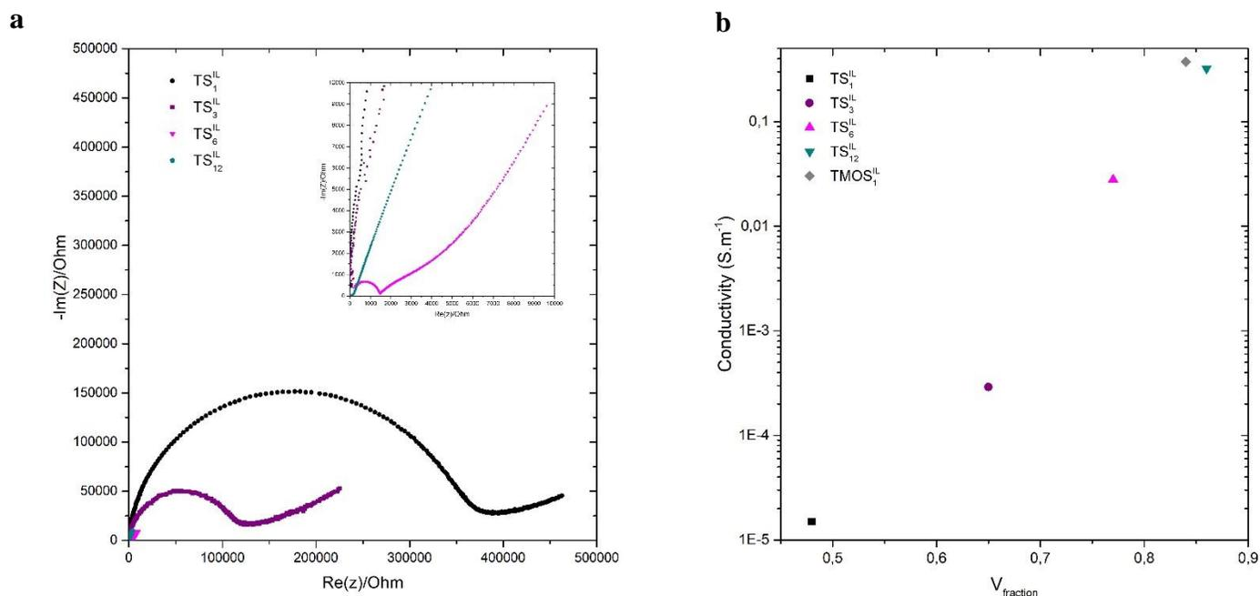
**Figure 7.** (a) Nyquist plots obtained for the different  $\text{TS}_x^{\text{IL}}$  samples using broadband dielectric spectroscopy (BDS), (b) the variation of the conductivity of the  $\text{TS}_x^{\text{IL}}$  and  $\text{TMOS}_1^{\text{IL}}$  materials as function of the IL  $V_{\text{fraction}}$ .
