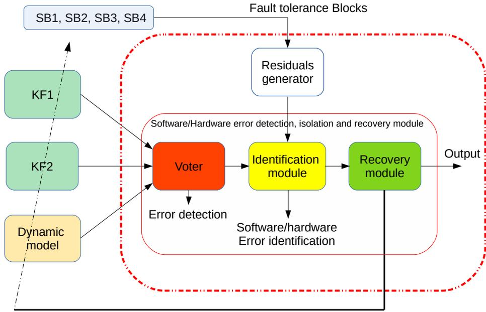
Figure 12: Software/hardware error detection, isolation and recovery module
