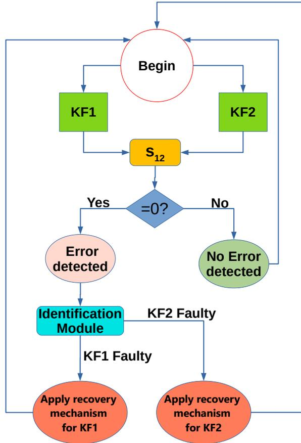
Figure 13: Proposed data fusion architecture for tolerating sensors and software faults
