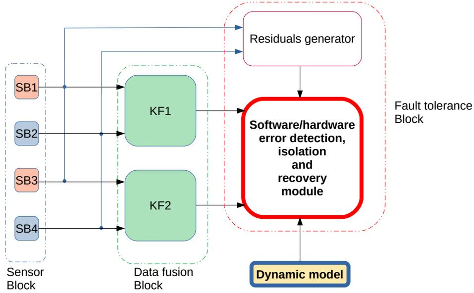
Figure 11: Fault tolerance architecture using Duplication comparison and analytical redundancy
