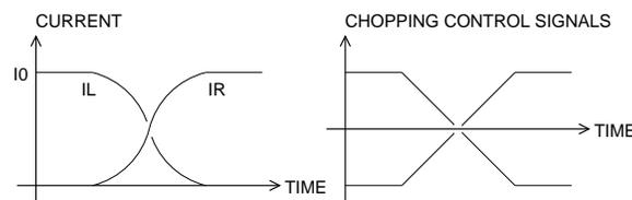
Fig. 10. Smooth switching of the biasing current
