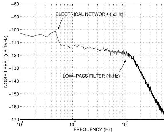
Fig. 15. Noise spectrum of the chopped microsystem
