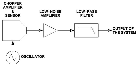
Fig. 11. Block diagram of the whole system
