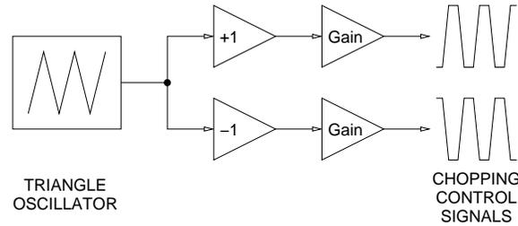
Fig. 9. Generation of the chopping control signals
