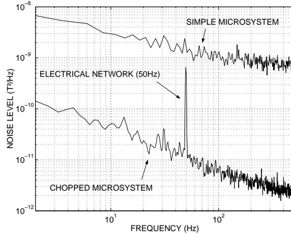
Fig. 14. Compared noise spectrums of the two microsystems
