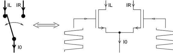
Fig. 8. The actual realization of the switches
