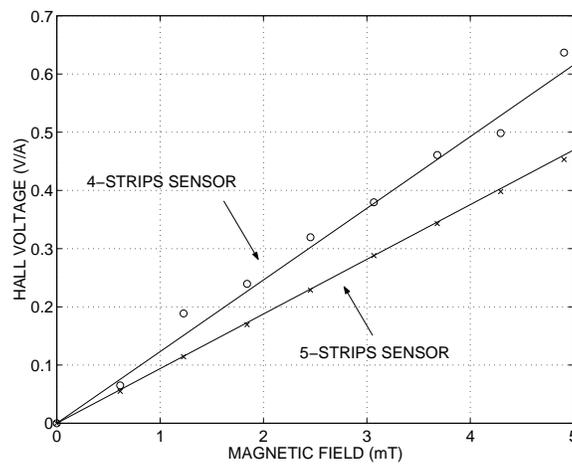
Fig. 13. Compared relative sensitivity of the two sensors
