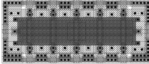
Fig. 12. Layout of the five strips Hall effect sensor ( $49.8 \times 21.4 \mu\text{m}^2$  including the  $\text{P}^{++}$  guard-ring, the size of the active area is  $39 \times 9.2 \mu\text{m}^2$ )
