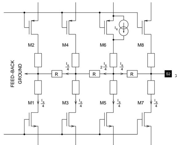
Fig. 6. Noise generated by the resistive coupling of the output stages
