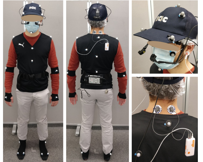
Fig. 3: Sensors setup: 27 motion capture markers, EMR eye-tracker with cap and battery bag, Shimmer3 GSR+ sensor with earlobe for PPG measurement and single-use gel-type electrodes for GSR measurements.
