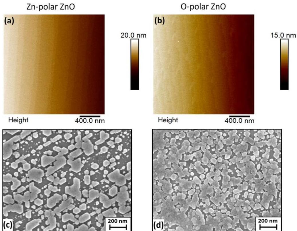
**Fig. 7** Top-view AFM images showing the topography of (a) Zn-polar and (b) O-polar ZnO single crystals. Top-view FESEM images of ZnO nuclei grown on the (c) Zn-polar and (d) O-polar ZnO single crystals.
