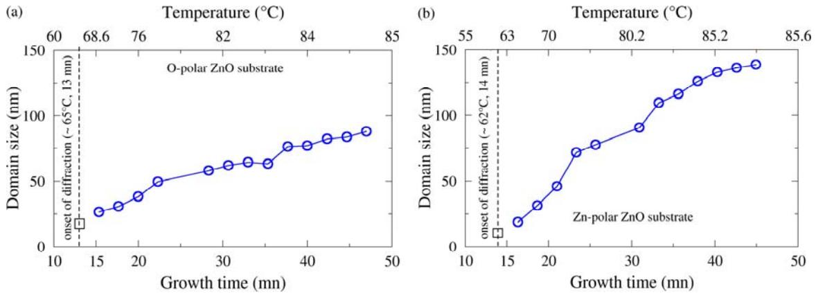
**Fig. 3** Evolution of the in-plane size of ZnO nuclei grown on the (a) O- and (b) Zn-polar ZnO single crystals, respectively, as a function of the growth time and temperature. The values of the in-plane size were deduced from the FWHMs of the Bragg peaks in the in-plane rocking scans presented in Fig. 2.
