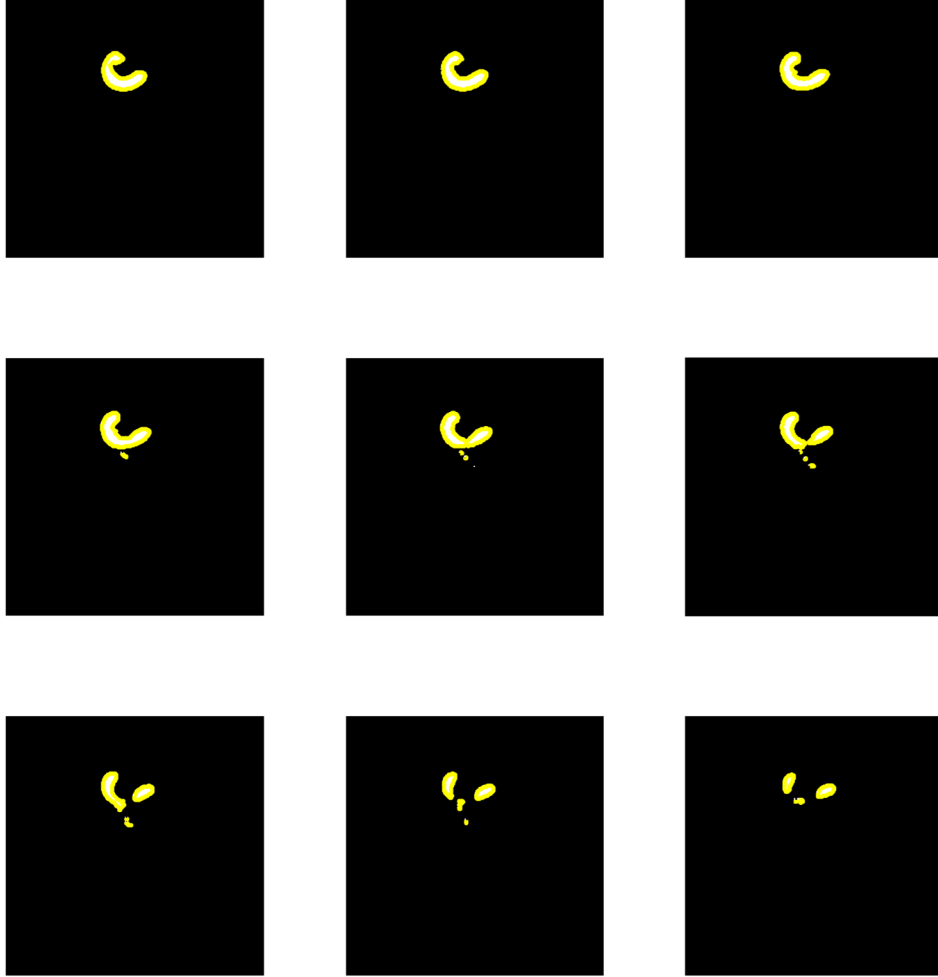
Fig 3. Illustration of region growing algorithm evolution with the automatic bifurcation points management.
