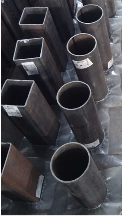
(a) Steel tubes prepared for casting
