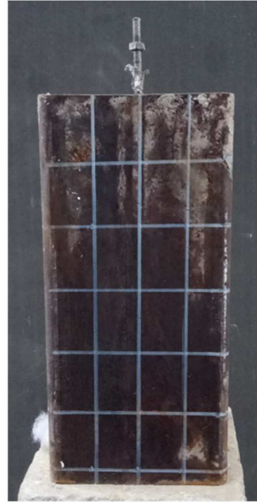
(c) CFST columns for the push-out tests
