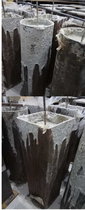
(b) CFST columns after casting
