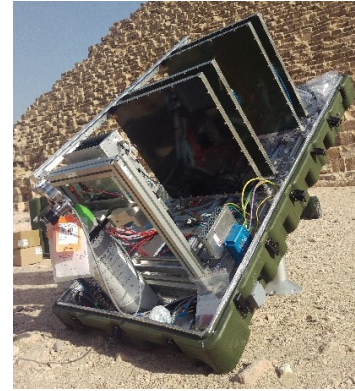
Figure 1: Photograph of one of the micromegas-based muon telescopes in use for muon tomography measurements. Details about their features and operation can be found in Refs. [19] and [20].
