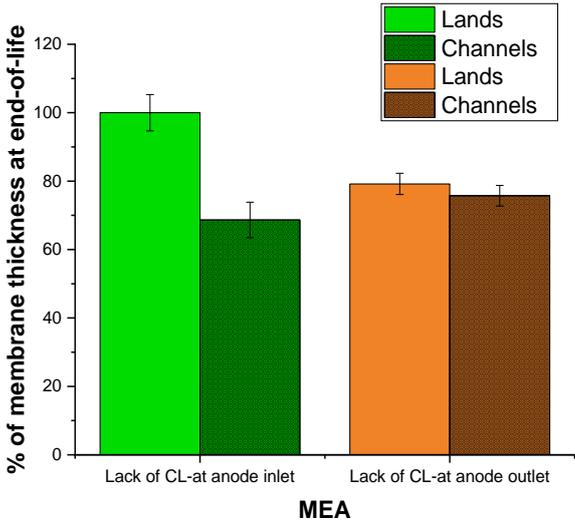
**Figure 7.** EoT membrane thickness compared to BoL (100%), below the channels and below the lands, in the segments with a lack of anode CL (i.e. #3 in the case of the MEA with a lack of anode CL near the hydrogen outlet, and #18 in the case of the MEA with a lack of anode CL near the hydrogen inlet). Data plotted on the graphs correspond to the average values of five measurements, with standard deviation.
