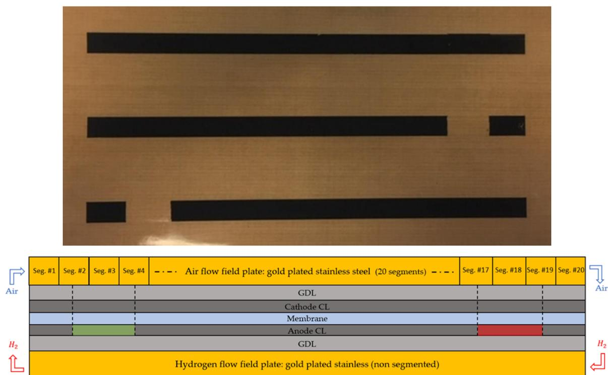
**Figure 2.** Up: anode -before transfer on the membrane- with -or without- a lack of CL at one end. Below: longitudinal sectional view of the segmented cell. The location of the defect is situated either at the anode inlet (in green) or outlet (in red).
