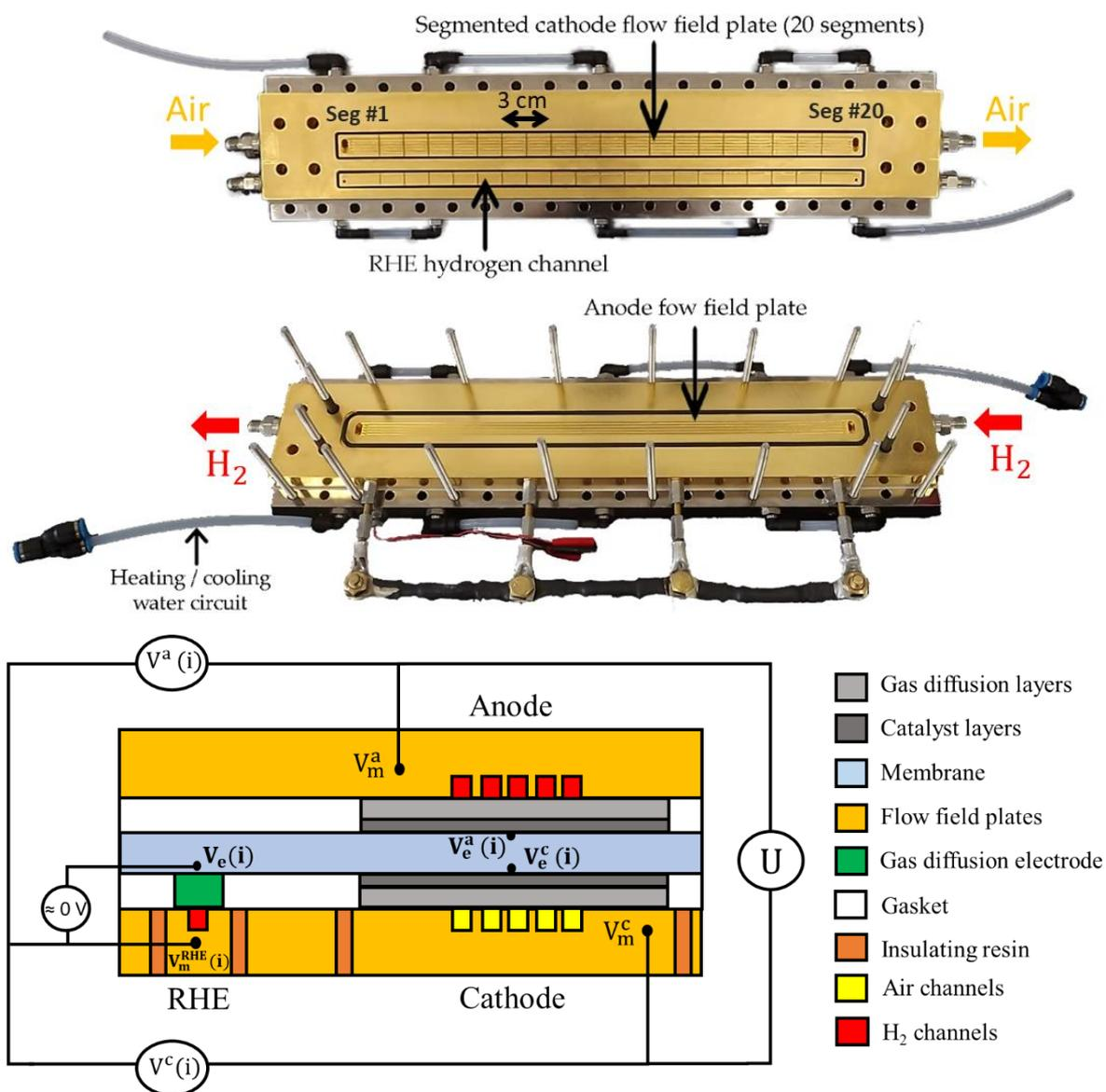
**Figure 1.** Pictures and operation principle of the linear segmented cell. Up: segmented cathode flow-field with the auxiliary hydrogen channel feeding the RHE used to measure the local potentials. Middle: anode flow-field plate. Bottom: cross-sectional view of the cell. The reference electrodes give access to the local electrolyte potential  $V^e(i)$  and thus to the anode and cathode potentials of each segment [22,35].
