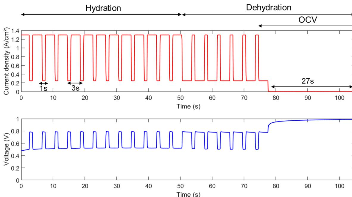
**Figure 3.** Current density and voltage profiles during the RH and load cycling AST. The hydration stage consists of alternating 1 s at low current (0.25 A/cm<sup>2</sup>) and 3 s at high current (1.3 A/cm<sup>2</sup>) sequences and lasts 52 s. The dehydration stage consists of alternated sequences of 3 s at low current and 1 s at high current, followed by 27 s at OCV (total duration = 105 s) [22].
