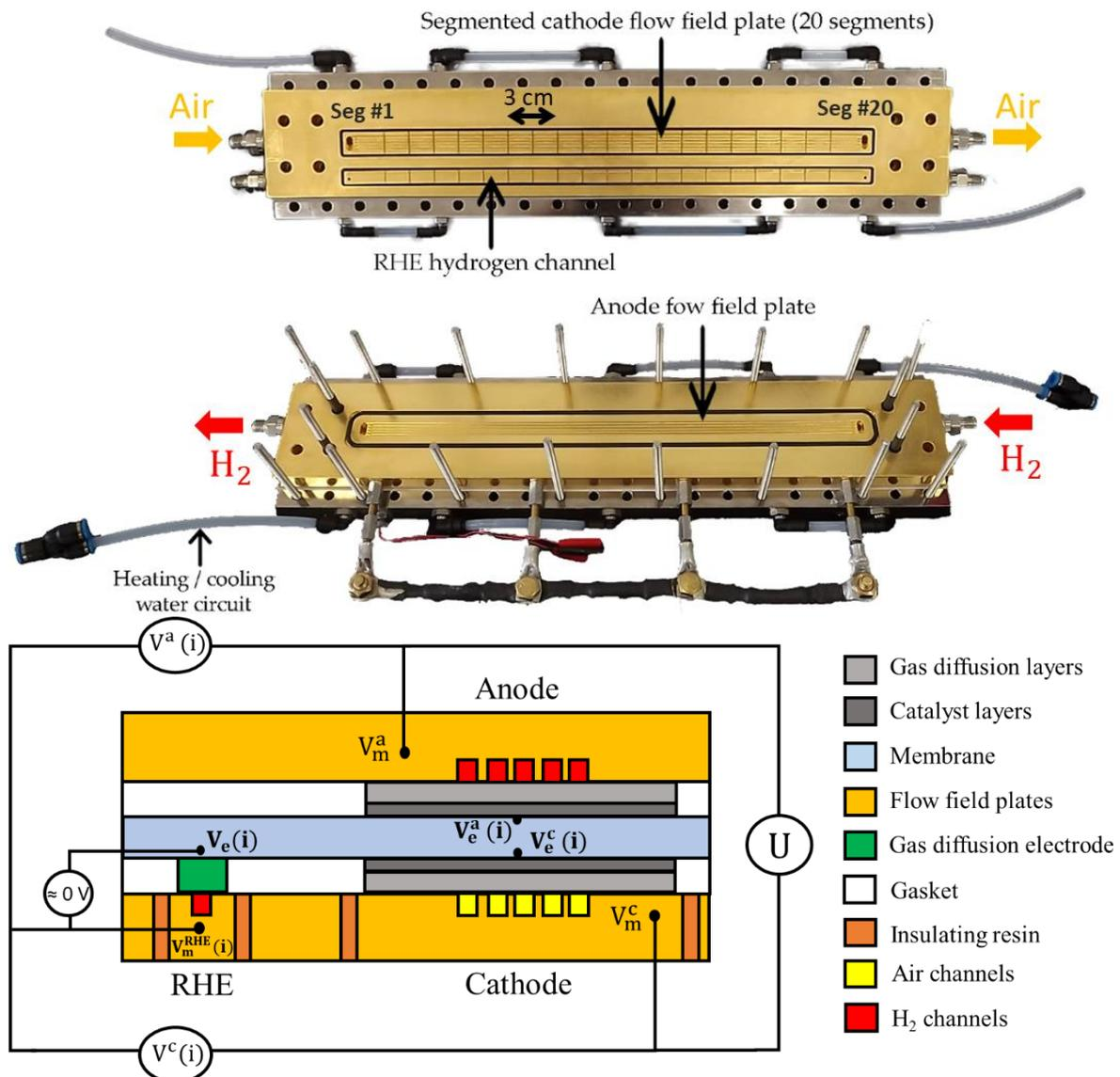
**Figure 1.** Pictures and operation principle of the linear segmented cell. Up: segmented cathode flow-field with the auxiliary hydrogen channel feeding the RHE used to measure the local potentials. Middle: anode flow-field plate. Bottom: cross-sectional view of the cell. The reference electrodes give access to the local electrolyte potential  $V_e(i)$  and thus to the anode and cathode potentials of each segment [22,35].
