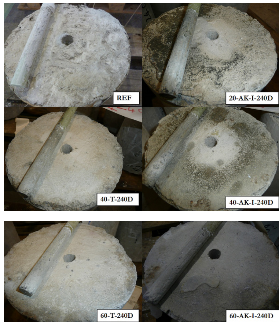
Figure 19. Typical failure modes observed after pull-out tests on reference and aged specimens.
