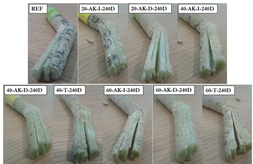
Figure 16. Failure modes observed after short-beam tests on reference and aged GFRP rebars.
